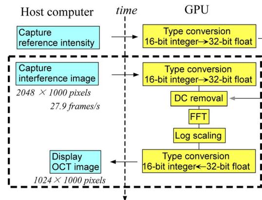
Fig. 3 Flowchart of real-time OCT imaging. The dashed block shows the routine procedure in our system.
