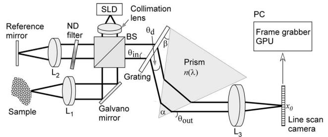
**Fig. 1** Schematic of spectral domain optical coherence tomography with a linear-in-wave-number spectrometer. SLD, superluminescent diode; BS, beamsplitter; L, achromatic lens;  $\theta_d$ , diffraction angle;  $\theta_{in}$ , incident angle;  $\theta_{out}$ , output angle of prism;  $\alpha$ , apex angle of prism;  $\beta$ , angle between grating and prism;  $x_0$ , central location of CCD camera.
