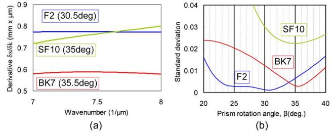
Fig. 2 Derivatives of the location of the spectral component at the optimal angle  $\beta$  with respect to wave number. (b) Standard deviation of derivatives with respect to angle between the prism and the grating.
