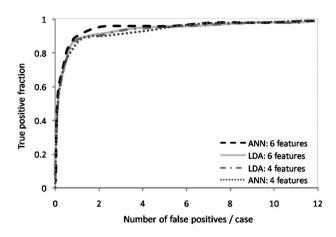
Fig. 6 FROC curves for the NFLD detection results by using the LDA and ANN with four and six image features.
