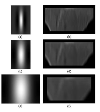
**Fig. 5** Filter kernels of the Gabor functions with different parameters: (a) filter size of  $41 \times 61$  with standard deviations of Gaussian function,  $\sigma_x = 6$  and  $\sigma_y = 15$ , (c) filter size of  $41 \times 61$  with  $\sigma_x = 12$  and  $\sigma_y = 20$ , and (e) filter size of  $81 \times 61$  with  $\sigma_x = 24$  and  $\sigma_y = 36$ . (b), (d), (f) Filtered output images corresponding to (a), (c), and (e), respectively.
