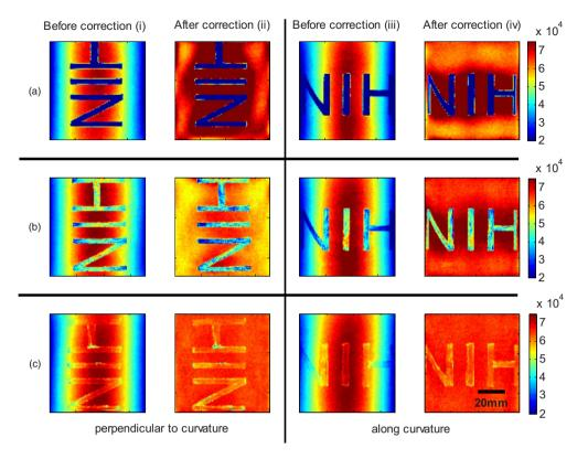
**Fig. 8** Curvature correction based on curve fitting on the cylindrical phantom with data (letters). Intensity images are shown before and after curvature correction. Different contrast agents were used with decreasing data-to-background ratios. The different  $I_d/I_b$  ratios are (a) 0.73, (b) 0.51, and (c) 0.39. The figure qualitatively shows the dependence of data-to-background ratio on the correction performance.
