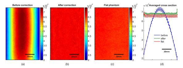
**Fig. 7** Curvature correction based on curve fitting on the cylindrical phantom without data content and compared to the flat phantom. (a) shows the curvature uncorrected intensity image, (b) the curvature corrected intensity image, and (c) shows the flat phantom. (d) shows the averaged cross section of (a), (b), and (c) with error bars given by the standard deviation over all rows.
