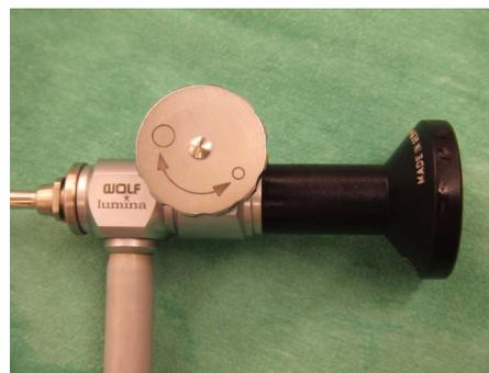
**Fig. 1** Magnification can be adjusted with a knob on the optical device (range 30 to 650 $\times$ ).
