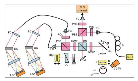
Fig. 1 Combined PS-OCT and SLO instrument for clinical imaging. Components: SLD, superluminescent diode; PC, polarization controller; FC, fiber coupler; POL, polarizer; PBS, polarizing beamsplitter; BS, nonpolarizing beamsplitter; QWP, quarter-wave-plate; GS, galvanometer scanner; L, lens; M, mirror; ND, variable neutral density filter; DC, dispersion compensation; RM, reference mirror; HWP, half-wave plate; DG, diffraction grating; LSC, line-scan camera; and CCTV, camera for pupil observation.
