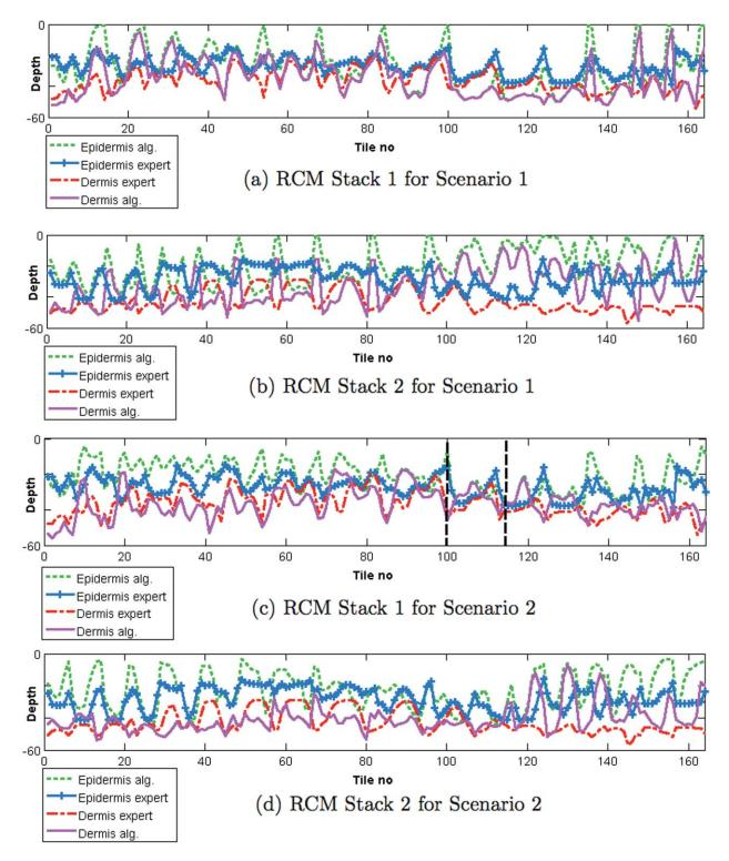
**Fig.** 7 For scenario 1 and 2 and RCM stacks 1 and 2, the figure show the epidermis and dermis boundaries located by the algorithm in comparision to the expert located boundaries for all of the 164 tile-sequences that were processed by the algorithm. The boundaries shown are 2D Gaussian filtered for smoothness as explained in the post-processing step in Sec 2. The dotted vertical lines in (c) indicate the location of the vertical slice shown in Fig. 8(b). (Color online only.)
