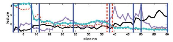
**Fig. 4** An example multivariate *z*-sequence of features. For illustration purposes, only four features are shown. The segment boundaries of the eight segments found by the sequence segmentation algorithm are shown with solid blue vertical lines. The dashed vertical red lines show the epidermis and dermis boundaries located by the expert. (Color online only.)
