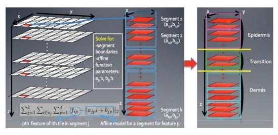
Fig. 5 Left panel shows the tile sequence and an example output of the sequential segmentation algorithm. Right panel shows the resulting epidermis and dermis boundaries (yellow longer horizontal lines) of the combined sequential+classification decision algorithm. (Color online only.)
