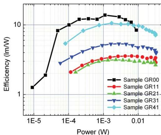
Fig. 9 Efficacy versus iLED power for different phosphor weight ratios.
