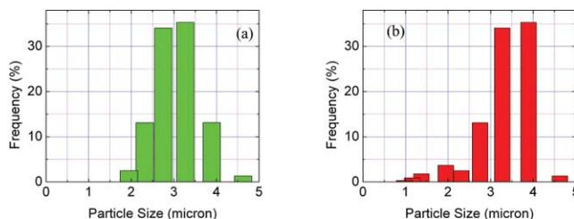
**Fig. 3** Particle size distributions of (a) PG phosphor and (b) PR phosphor as determined by dynamic light scattering.
