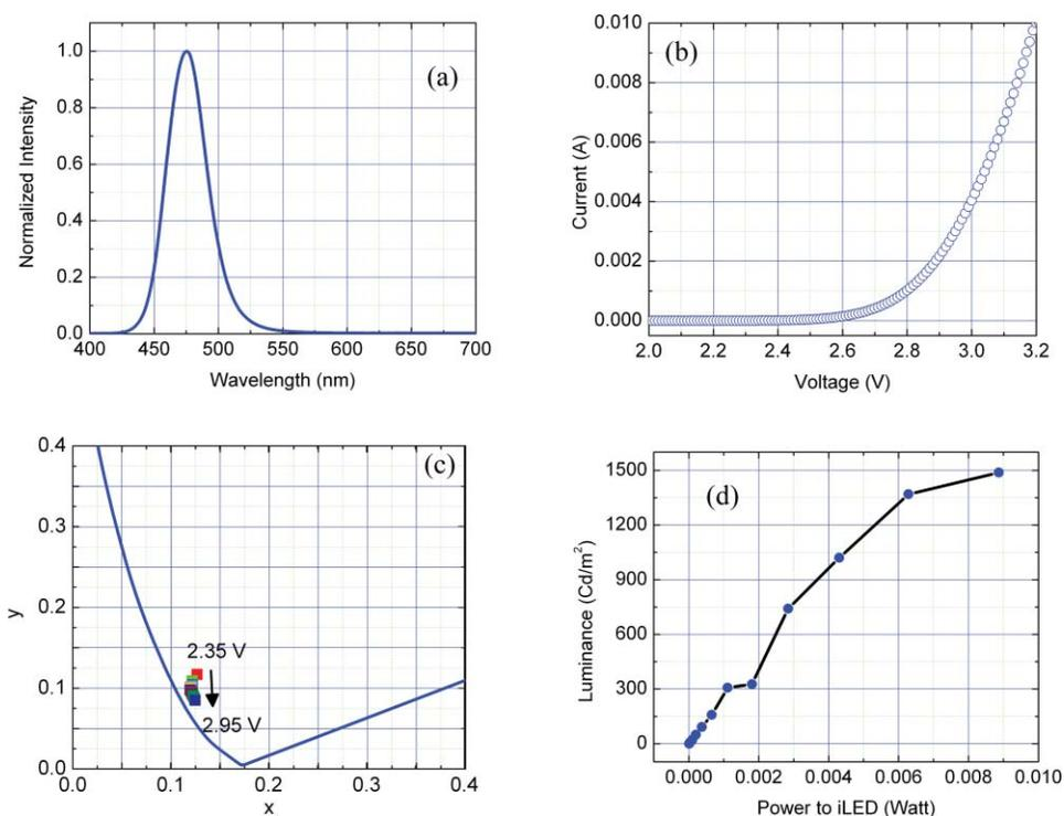
**Fig. 1** (a) Electroluminescent spectra from an iLED at 2.4-V driving voltage, (b)  $I$ - $V$  characteristics of a typical iLED, (c) expanded 1931 CIE diagram showing the shift of the CIE coordinates versus voltage to the iLED, and (d) luminance versus power of iLED.
