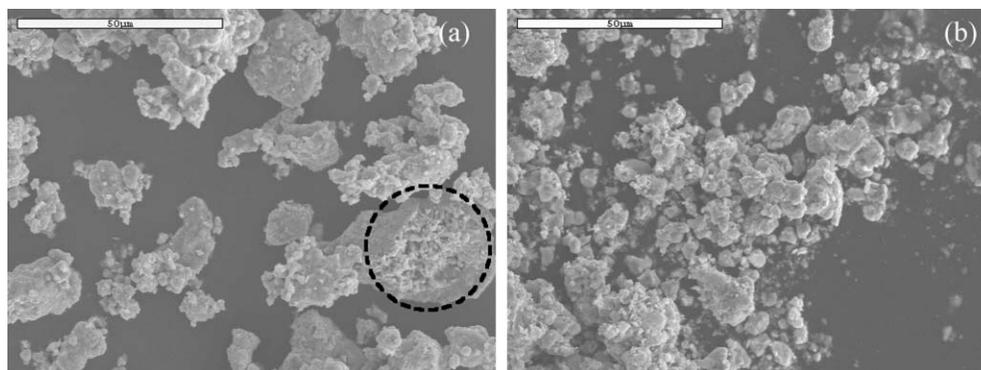
**Fig. 4** SEM images of dried (a) green-emitting phosphor (PG) and (b) red-emitting phosphor (PR). The dotted circle in (a) shows that the large agglomerated particles are composed of small particles. (Scale bar: 50  $\mu\text{m}$ ).
