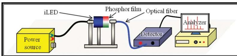
**Fig. 2** Instrumental setup for photoluminescence measurement.
