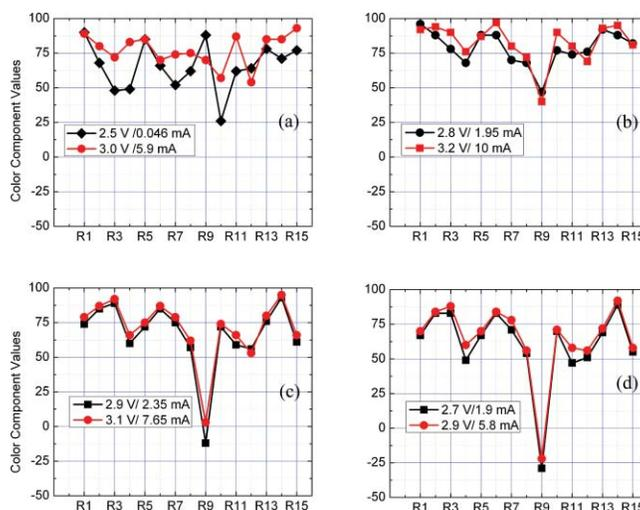
**Fig. 8** Color-rendering index values of R1-R15 standard colors for sample (a) GR11, (b) GR21, (c) GR31, and (d) GR41. The maximum Ra value for GR11, GR21, GR31, and GR41 was 79, 86, 78, and 74, respectively.
