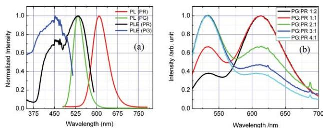
**Fig. 5** (a) PL and PLE spectra from PG and PR phosphors and (b) PL spectra from mixtures of green and red phosphors (PG and PR). Legends show the weight ratio of green to red phosphors.
