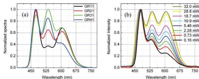
**Fig. 6** (a) Normalized downconversion emission spectra of thin-film samples prepared using various weight ratios of PG to PR phosphors in a PMMA host at 4 mA. (b) Normalized downconverted white light from the sample PG21 versus power to the iLED.
