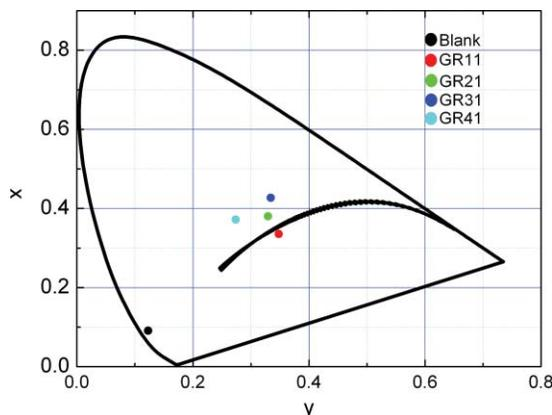
**Fig. 7** Color coordinates of downconverted white light from samples with different weight ratios of green to red phosphors.
