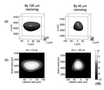
**Fig. 10** (a) -6 dB isosurface of a 3-D PA image of a 50- $\mu$ m bead. (b) A 2-D image on the plane crossing the central position of the bead displayed over a 10-dB dynamic range.
