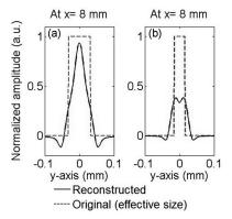
**Fig. 4** Simulated 1-D PAT profile along y of (a) 100- and (b) 50- $\mu$ m PS beads at position C using 60- $\mu$ m microring detectors.
