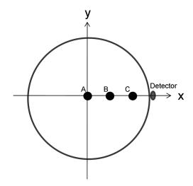
Fig. 1 Diagram of beads positions and scanning geometry in PAT experiments.
