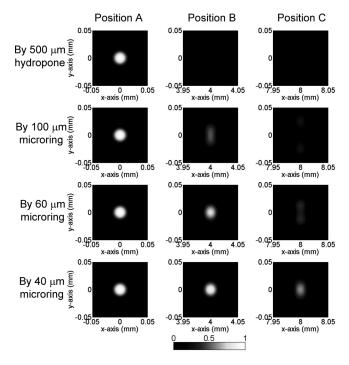
**Fig. 3** Simulated PAT images of  $50-\mu m$  PS beads (effective size =  $31 \mu m$ ) using different types of detectors.
