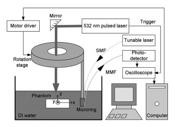
**Fig. 6** Experimental setup of PAT imaging (SMF: single-mode fiber; MMF: multi-mode fiber).
