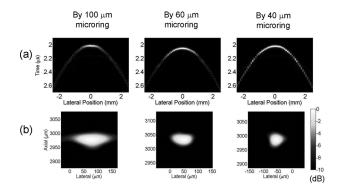
**Fig. 9** (a) Wave field plot of the detected acoustic field along a 1-D array and (b) reconstructed image of the cross section of a  $6-\mu$ m-diameter carbon fiber displayed over a 10-dB dynamic range, where 0 dB represents the maximum reconstructed signal.
