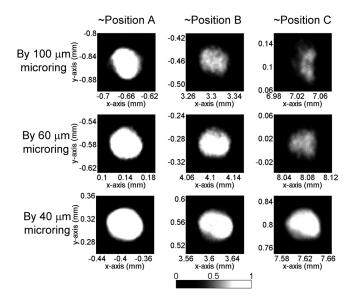
Fig. 7 PAT images of 100- $\mu$ m PS beads (effective size = 62  $\mu$ m) using microrings.
