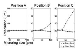
**Fig.** 5 Simulated spatial resolution of 50- $\mu$ m beads imaged by different microring size at positions A, B, and C.
