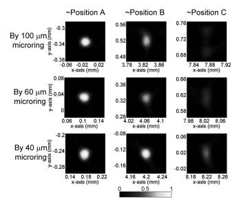
**Fig. 8** PAT images of 50- $\mu$ m PS beads (effective size = 31  $\mu$ m) using microrings.
