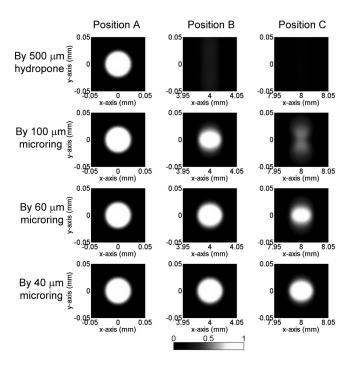
**Fig. 2** Simulated PAT images of 100- $\mu$ m PS beads (effective size =  $62~\mu$ m) using different types of detectors.
