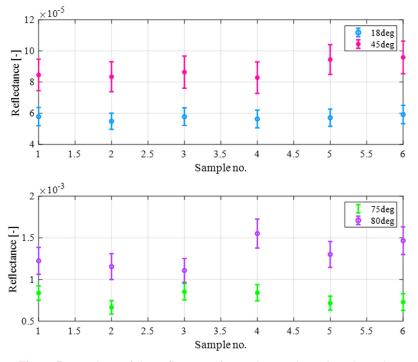
Fig. 4 Raw values of the reflectance for each sample and each angle.
