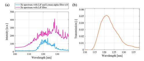
**Fig. 2** (a) The comparison of the Xe plasma spectrum measured with the LiF filter (pink line), and the spectrum measured with additional Lyman- $\alpha$  filter (blue line). Note that the Xe plasma spectrum with the Lyman- $\alpha$  filter has been multiplied by 10 to better visualize the difference between both spectra. (b) The transmission of the Lyman- $\alpha$  filter used in the reflectance measurements.
