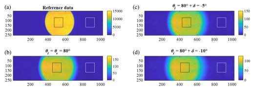
**Fig. 5** Reflectance raw data taken for xenon: (a) reference data and (b) examples of the data taken for the incidence angle  $\theta_i = 80$  deg for specular reflection, and for off-specular case (c) at  $\theta_i = 80$  deg,  $\delta = -5$  deg, and (d) at  $\theta_i = 80$  deg,  $\delta = -10$  deg. Note the intensity change indicated by the colorbar.
