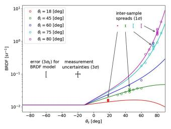
Fig. 11 Comparison of BRDF measurement data for the UV regime ~121.6 nm (circles) with the best globally fitted model (solid lines). The error bars for the mean error of the fit, measurement uncertainties, and inter-sample spreads are shown in the plot. Different colors represent different incidence angles.
