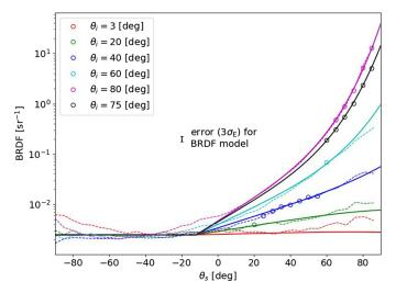
**Fig. 8** BRDF measurement data for 532 nm (dashed lines), from which a limited subset *S* of data points (circles) was selected for pre-validation of fitting procedures used later for ~121.6 nm. The solid lines show the best globally fitted model for 532 nm. The error bar for the mean error  $3\sigma_E$  of the fit is shown in the middle of the plot. Different colors represent different incidence angles.
