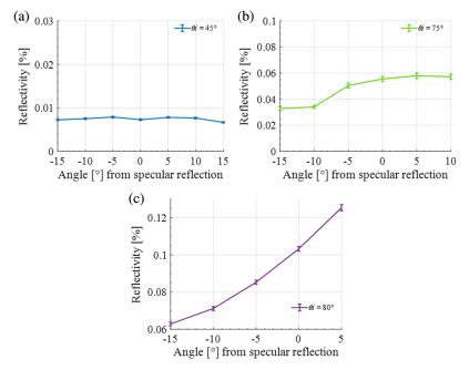
**Fig. 6** Results of the off-specular measurements for the incidence angles of (a)  $\theta_i = 45$  deg, (b)  $\theta_i = 75$  deg, and (c)  $\theta_i = 80$  deg.
