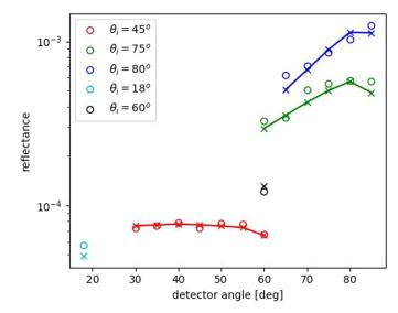
Fig. 14 Comparison of the measured (circles) and simulated (crosses) raw reflectance for series II of measurements in the UV regime discussed in Sec. 3. Different colors correspond to different incidence angles.
