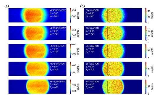
Fig. 13 Comparison of (a) measured CCD images registered in measurements discussed in Secs. 2 and 3 with (b) ray tracing simulations.
