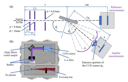
Fig. 1 A scheme of the experimental setup used in reflectance measurements: (a) with dimensions and visualization of the reference and angular measurements and (b) with a description of each component.
