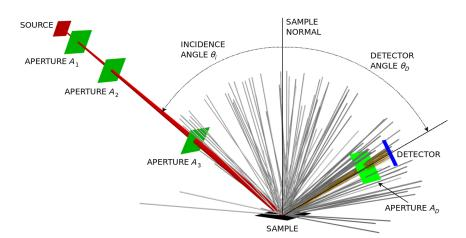
**Fig. 12** Schematic view of the simulation setup. The incident beam (shown in red) is formed by three apertures  $A_1$ - $A_3$  (green). Two types of rays scattered from the sample (black) are shown. Gray lines represent instances of rays scattered in random directions, and yellow lines show instances of scattered rays that were registered by the detector (blue). Between the sample and the detector, an additional aperture  $A_D$  is placed.
