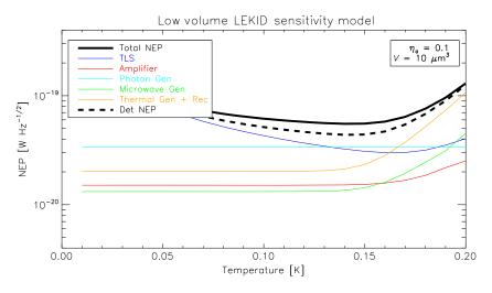
**Fig. 5** Sensitivity model predictions for the low volume LEKID proposed here, with  $\eta_a=0.1$ ,  $V_L=10~\mu{\rm m}^3$ , and maximized  $P_g$  (see text for details). Detector NEP (black dashed) includes all contributions to the NEP aside from the photon generation noise. The optimal operating temperature is  $T\approx 150~{\rm mK}$ .
