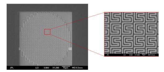
**Fig. 7** Photograph of the inductor/absorber portion of a 10- $\mu$ m LEKID. The inset shows the basic unit cell, optimized for the absorption of vertically polarized radiation, replicated over the full 60- $\mu$ m diameter absorber area. Simulations indicate a peak single-polarization absorption efficiency of 70% near 10  $\mu$ m. Figure duplicated unaltered from Ref. 70; license can be found at Ref. 72.
