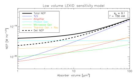
**Fig. 6** Same as Fig. 5 with T=150 mK. With an optical load of  $P_o=10^{-18}$  W, the photon generation noise is NEP<sub>photon</sub> =  $3.4\times10^{-20}$  W Hz<sup>-1/2</sup>, and the detector noise with  $V_L=10~\mu\text{m}^3$  is NEP<sub>det</sub> =  $4.4\times10^{-20}$  W Hz<sup>-1/2</sup>. Further reductions in the detector NEP are possible by further reducing  $V_L$ .
