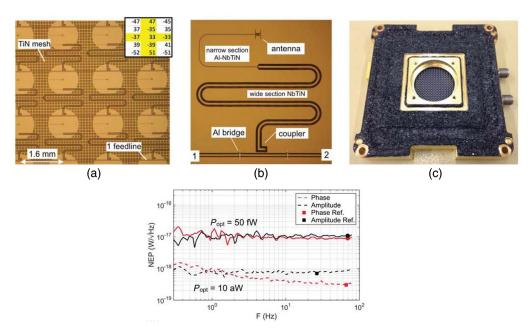
**Fig. 2** SPACEKIDs detector figures from Ref. 2. Top: Photographs of the 961 pixel demonstration array highlighting (a) the TiN absorbing mesh located between the detector wafer and lens array, (b) the quarter-wave CPW hybrid NbTiN-Al KID and the coupled twin-slot antenna, and (c) the fully assembled detector package. Bottom: Measured NEP of a representative detector for phase and amplitude readout. Credit: Ref. 2, reproduced with permission © ESO.
