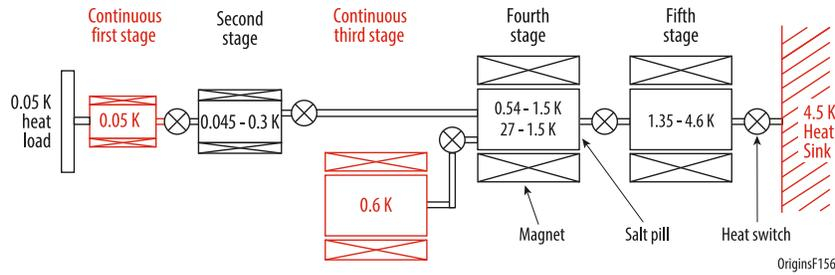
**Fig. 7** The FIP CADR provides continuous cooling at two stages: 50 mK (with 0.4  $\mu$ K stability) and 0.7 K (with 0.1 mK stability), and deposits its heat at a 4.5 K heat sink.
