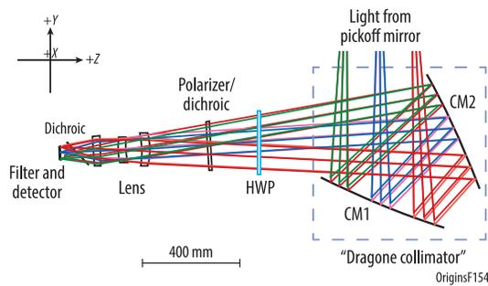
**Fig. 5** The FIP optical system minimizes the number of optical components. This configuration shows the layout for a polarization measurement because the HWP is in the beam.
