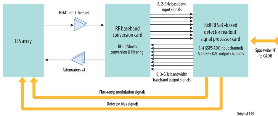
**Fig. 6** Detector readout scheme for FIP: FIP and RFSoc samples and processes signals simultaneously
