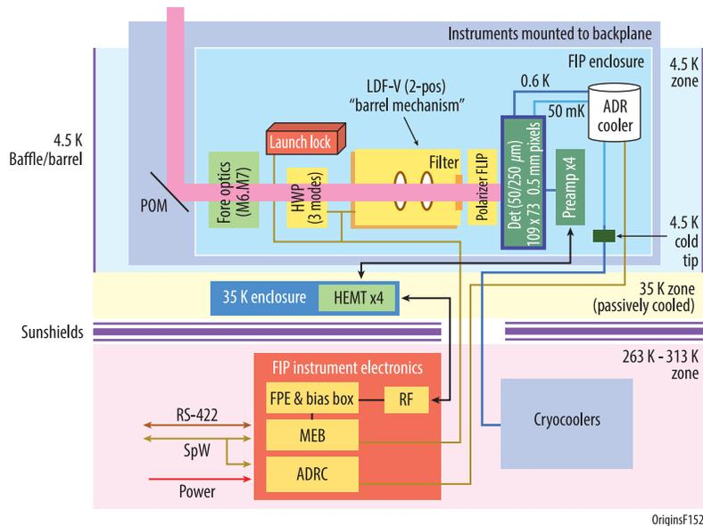
**Fig. 3** FIP has a simple design with one detector selectable by filter to 50 or 250  $\mu\text{m}$ . This functional block diagram of FIP shows how the power dissipation in the cold 4.5 K section is minimized by placing the readout electronics in the warm part of the observatory.
