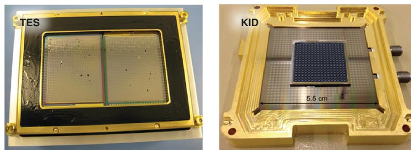
**Fig. 2** The Origins Technology Development Plan recommends parallel investment in two detector technologies for FIP: TES bolometers and KIDS.
