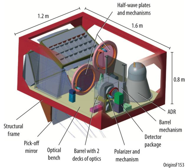
**Fig. 4** The FIP mechanical structure and components. The labels point out individual components described in the text.
