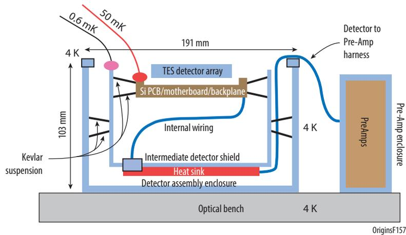
**Fig. 8** The FIP focal plane array is cooled to 0.05 K and suspended within a 0.7 K enclosure, providing thermal shielding from the 4.5 K stage. The Kevlar suspension, which is common to most instruments with low temperature detectors, provides for excellent stiffness while having a very low heat conductivity.
