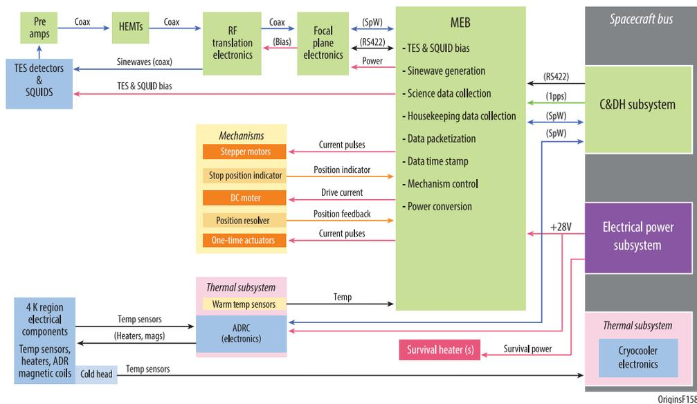
**Fig. 9** This FIP block diagram shows how the instrument is controlled.
