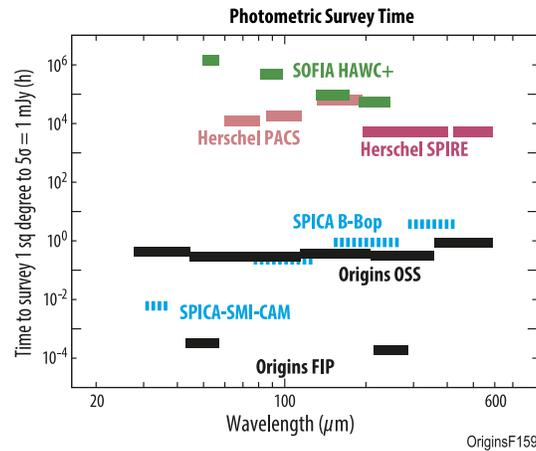
**Fig. 10** A comparison of photometric survey times for a number of space-based FIR instruments. It is worthy to note that Origins/FIP will be the fastest mapping far-IR survey instrument ever.
