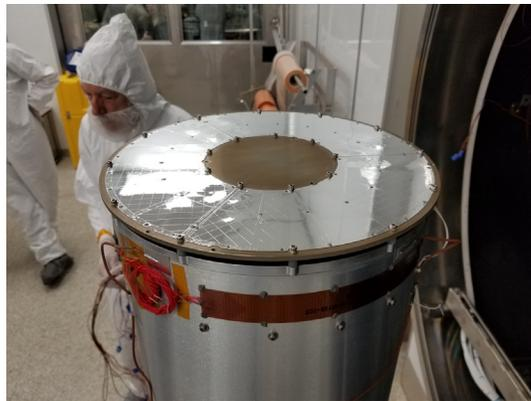
**Fig. 6** A thermal shield mounted on the rear of a flight mirror module assembly. Visible just below the shield is a band heater (one of three at each end) that maintains the MMA within its operating temperature range.
