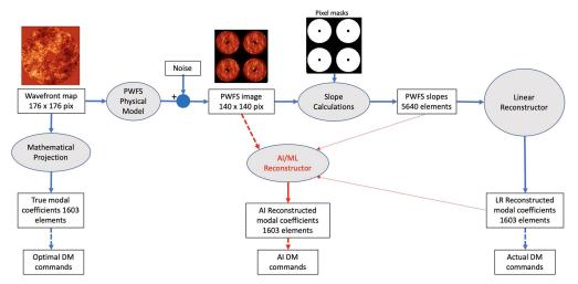
Fig. 1 Outline of the simulation pipeline. Thin red-dotted lines are possible inputs to the ML model that we did not pursue in this work. The thick red lines show the inputs and outputs of the proposed ML model.
