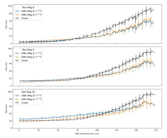
**Fig. 8** Wavefront reconstruction quality as a function of RMS for magnitudes 8, 9, and 10. Models were trained on either magnitude 8 or 9 data with an f-value of p = 2 power law. Moving averages are plotted to help visualize the trend, with error bars showing one standard deviation for that window.
