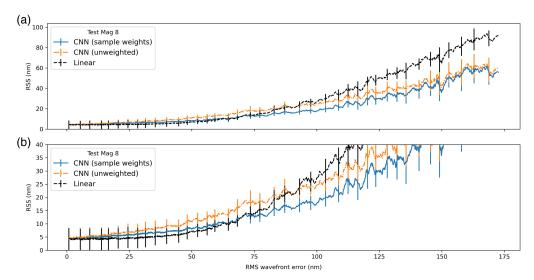
**Fig. 5** Weighting samples by RMS value improves model performance. (a) The overall change and (b) a zoomed-in view of the lower (<125 nm) RMS cases. Samples were weighted based on their RMS, with low RMS samples being higher weighted. Moving averages are plotted to help visualize the trend, and error bars are the standard deviation of the window.
