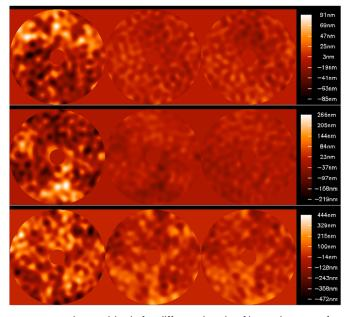
**Fig. 6** Wavefront reconstruction residuals for different levels of incoming wavefront. Left: incoming wavefront map, 400 KL modes (30/80/134 nm RMS). Middle: residual wavefront error map after linear reconstruction (8/25/85 nm RMS). Right: residual wavefront error map after CNN reconstruction (10/19/69 nm RMS).
