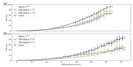
**Fig. 12** Error by RMS of two models trained on different f-values. (a) Models reconstructing  $f^{-1.8}$  samples and (b) reconstructing  $f^{-1.8}$  samples. Moving averages are plotted to help visualize the trend. Error bars are one standard deviation for that window.
