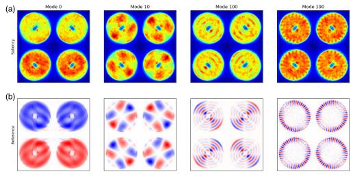
**Fig. 10** Selection of modes comparing saliency and idealized Karhunen–Loève modes. (a) The importance of each pixel to the model when determining the modal output. (b) The corresponding Karhunen–Loève mode.
