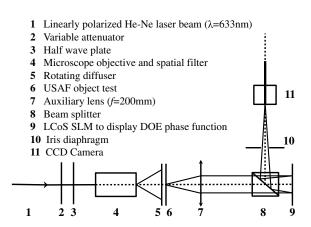
**Fig. 5** Experimental setup to evaluate the extended depth of field/focus of programmable DOEs.
