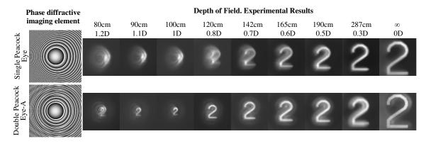
**Fig. 6** Experimental depth of field for two peacock eye-based elements. With an aperture of 8.64 mm (display size), the f-number (F/#), and the numerical aperture (NA) for some object positions within the depth of field are: object at infinity, F/# = 75; object at 142 cm, NA =  $3.0 \times 10^{-3}$  and object at 90 cm, NA =  $4.8 \times 10^{-3}$ ).
