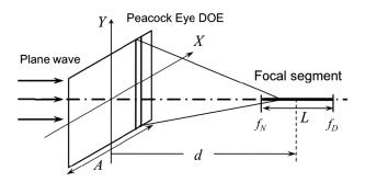
Fig. 1 Geometrical scheme of the design of the peacock eye element.
