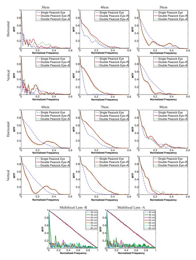
Fig. 4 Experimental MTFs computed from the results of Fig. 3.
