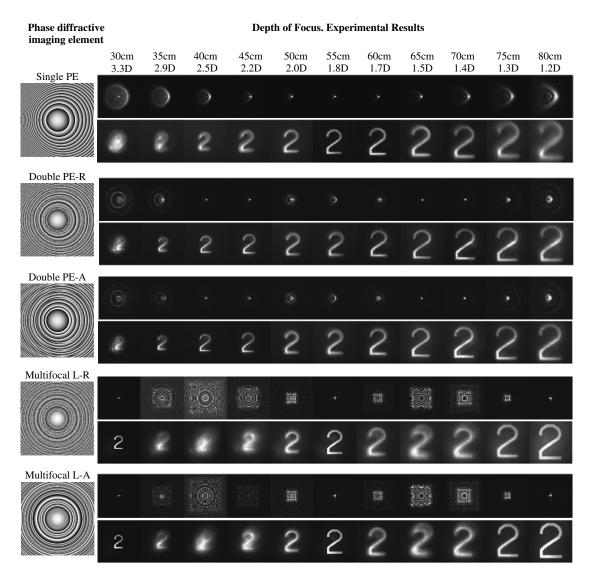
Fig. 3 Experimental PSFs and images of an extended object along different positions of the focal segment obtained with the phase diffractive elements represented in gray levels on the left.
