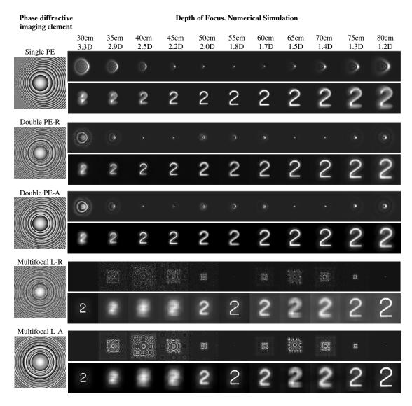
**Fig. 2** Numerical simulation of the PSFs and the images of an extended object along different positions of the focal segment obtained with the phase diffractive elements represented in gray levels on the left. PE stands for peacock eye, R for random, A for addition, and L for lens. With an aperture of 8.64 mm (display size), the f-number for the extremes and the center image positions of the focal segment are:  $f_N = 30$  cm, F/# = 35; f = 50 cm, F/# = 58 and  $f_D = 80$  cm, F/# = 93).
