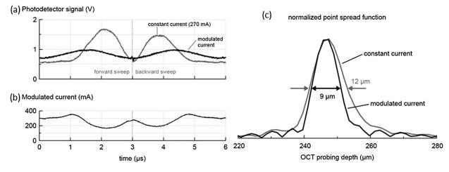
Fig. 2 Spectral shaping of forward and backward sweep of the FDML source: (a) Instantaneous power of forward and backward sweep at constant SOA current (gray trace) and at modulated SOA current (black trace); (b) modulated SOA current for spectral shaping; (c) resulting point spread functions with constant or modulated SOA current.
