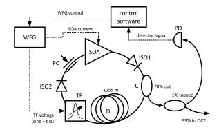
**Fig. 1** Set-up of FDML Source, SOA: semiconductor optical amplifier, FC: fiber coupler, DL: delay line, ISO: optical isolator, TF: tunable filter, PC: polarization controller, WFG: waveform generator, PD: photodetector.
