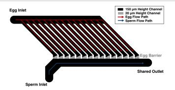
**Fig. 1** Top view of the microfluidic chamber. Eggs flow from the egg inlet toward the shared outlet through  $150-\mu$ m-height channels (black). Eggs reach smaller  $20-\mu$ m-height channels (gray) that are impassable and are immobilized. Sperm are flowed from the sperm inlet to the shared outlet and can be moved to eggs using optical trapping.
