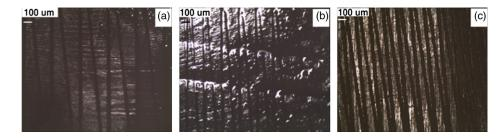
Fig. 2 Optical microscope images of fs-laser patterned teeth surfaces at 100 mW average laser power for (a) 20, (b) 30, and (c) 40 lines.
