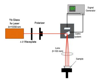
Fig. 1 Schematic setup for Fs-laser etching experimental procedure.
