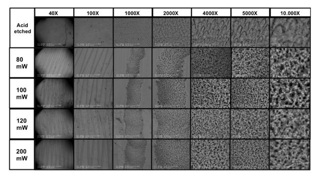
Fig. 5 SEM examinations were made for observing the irradiated enamel by an environmental scanning electron microscope. The recorded photos were grouped according to the laser power and magnification types.
