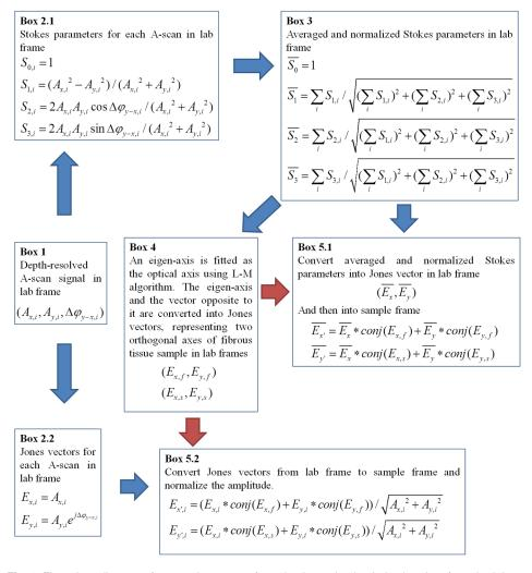
**Fig. 2** Flow chart diagram of processing to transform depth-resolved polarization data from the laboratory frame (LF) into the fibrous tissue sample frame (SF). Blue arrows indicate the data transformation, red arrows indicate that the fast and slow axes determined in Box 4 are applied in Boxes 5.1 and 5.2 for conversion from LF to SF, and *conj* refers to complex conjugate.
