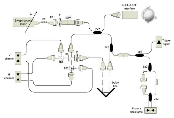
**Fig. 1** Clinical swept-source (SS) polarization-sensitive (PS) optical coherence tomography (OCT) system. PC: polarization controller; FP: fiber port; P: polarizer; EOM: broadband electro-optic modulator; BS: nonpolarization beam splitter; PBS: polarization beam splitter.
