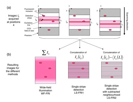
**Fig. 3** Description of the image processing methods. (a) Schematic of images taken at three different positions of the excitation line. (b) Processing method for each detection scheme;  $I_k(i)$ : intensity in line i of the image  $I_k$ ,  $i_d$ : detection stripe (located over the excitation line in this example), L: size of the neighboring area considered to calculate the background signal to subtract.
