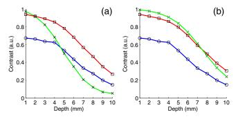
**Fig. 6** Comparison of the contrast obtained for a single fluorescent inclusion at 10 depths with the different methods with (a) basic parameters and (b) optimized parameters: WF-FRI (blue circles), LS-FRI1 (red squares), and LS-FRI2 (green x).
