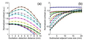
**Fig. 7** Contrast obtained with (a) LS-FRI1 versus excitation-detection distance D and (b) LS-FRI2 versus adjacent area size L for one fluorescent inclusion located at: 1 mm (dark blue circles), 2 mm (pink stars), 3 mm (light green x), 4 mm (solid black), 5 mm (yellow +), 6 mm (red squares), 7 mm (light blue diamonds), 8 mm (violet down triangle), 9 mm (blue triangle), and 10 mm (brown side triangle).
