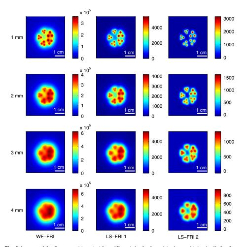
Fig. 9 Images of the fluorescent target at four different depths from 1 to 4 mm obtained with the three methods.
