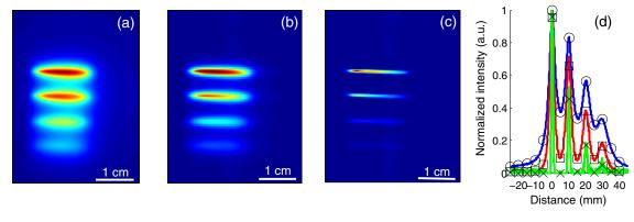
**Fig. 10** (a) Image obtained with WF-FRI; (b) Image obtained with LS-FRI1; (c) Image obtained with LS-FRI2 (top view); (d) Normalized intensity profiles obtained with: WF-FRI (blue circles), LS-FRI1 (red squares), and LS-FRI2 (green x); images (a), (b), and (c) are normalized.
