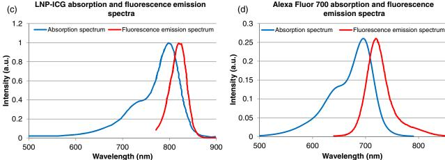
**Fig. 2** Physical characteristics of the complex phantoms studied [fluorescence resolution target (a) and phantom with four inclusions (b); Absorption and fluorescence emission spectra of LNP-ICG (c) and Alexa Fluor 700 (d)].
