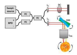
**Fig. 1** Schematic of the high-resolution 1060-nm swept-source optical coherence tomography system used to image the mouse hearts. The hearts were rotated about the long axis as shown. FC, wavelength-flattened fiber couplers; DC, dispersion compensation block; BDP, balanced photodiode detector; GM, galvanometer-scanning mirrors;  $L_C$ , collimating lens;  $L_{OBJ}$ , telecentric objective lens.
