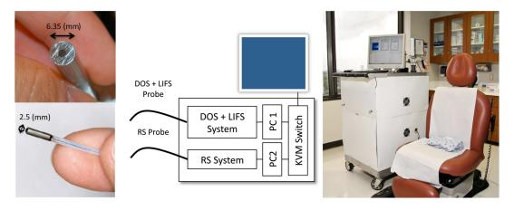
Fig. 1 Spectral diagnosis (SD) system in a clinical setting. It consists of two independent systems, each with a customized fiber optic probe. Details of the system are available in Sec. 2.
