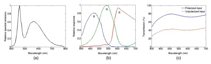
Fig. 2 (a) Relative emission spectrum of white light source, (b) relative spectral response of the 3-CCD, and (c) transmittance of the polarizer.
