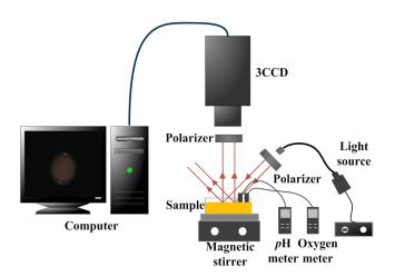
Fig. 1 Schematic of the color imaging system with devices measuring pH and dissolved oxygen in the sample. The red lines with arrows represent light flow.
