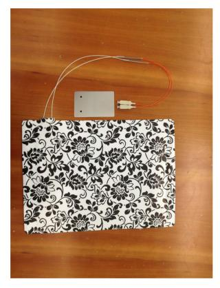
Fig. 10 Prototype system of the microbend fiber optic sensor mat and transceiver.
