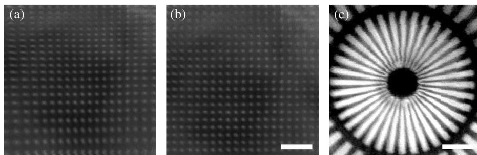
**Fig. 5** Reflection images of test targets (R1L3S5P, Thorlabs): (a) image of a distortion grid with the period of  $5 \mu\text{m}$ ; (b) reconstructed image of (a); and (c) reconstructed image of a Siemens star target with  $100\text{-}\mu\text{m}$  diameter center circle. Scale bar is  $20 \mu\text{m}$ .
