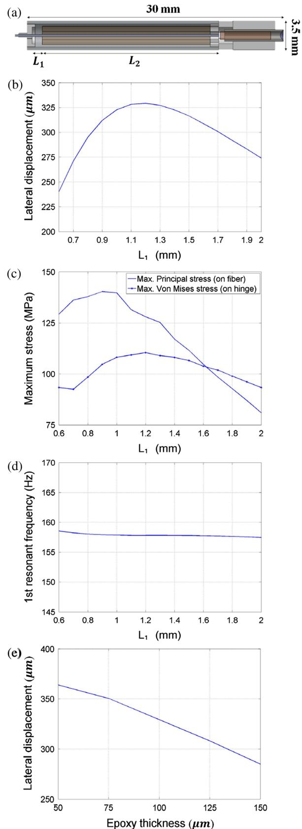
**Fig. 3** Finite element method simulation results: (a) the location of  $L_1$ ,  $L_2$  (21 mm, fixed); (b) lateral displacement according to  $L_1$ ; (c) maximum stresses on fiber and hinge according to  $L_1$ ; (d) the first-resonant frequency of fiber according to  $L_1$ ; and (e) lateral displacement according to the thickness of the epoxy bonded between the fiber and the hinge.
