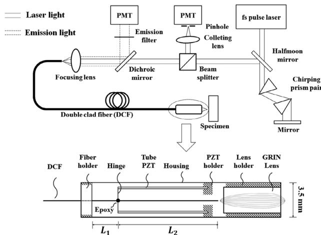
**Fig. 1** The system configuration of the raster scanning two-photon endomicroscope.
