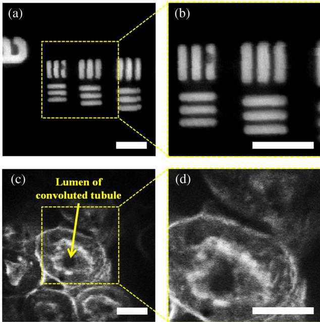
**Fig. 7** (a) The image of 1951 USAF test target (group 7, element 4, 5, and 6); (b) two times magnified image of (a) obtained by partial scanning; (c) the image of mouse kidney section; and (d) two times magnified image of (c) obtained by partial scanning. The lumen of the convoluted tubule is marked with yellow arrows. Scale bar is 20  $\mu\text{m}$ .
