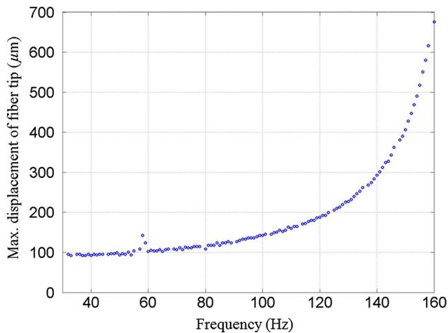
**Fig. 4** Frequency response of the assembled endomicroscope is described. Sinusoidal voltage with the amplitude of  $\pm 50$  V was driven to the fast axis piezoelectric actuators. The frequency was varied from 32 to 160 Hz.
