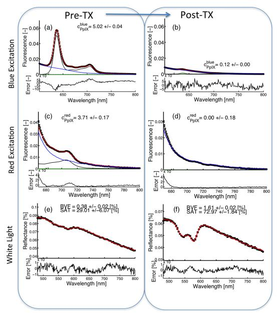
**Fig. 7** Representative optical measurements of fluorescence emission with excitation with (top) blue, (middle) red, and (bottom) white light reflectance from patient ID1. Left-hand panels show measurements 1 h following aminolevulinic acid administration (pre-Tx). Right-hand panels show measurements immediately after administration of treatment light (post-Tx).
