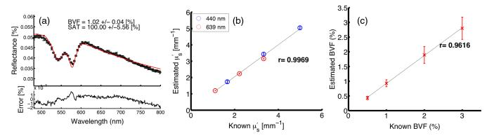
Fig. 4 (a) Representative white light spectra sampled in tissue phantoms for Intralipid 1% and blood volume of 1%. Estimated versus known values for (b) reduced scattering coefficient at blue and red excitation wavelengths and (c) blood volume fraction. Error bars on (b) and (c) represent variation between phantoms.
