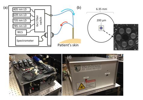
**Fig. 1** (a) Schematic of the multichannel dosimeter setup showing system components. (b) Fiber arrangement of the patient-interface (probe tip), which is used in light compression contact-mode. The source fiber is represented in blue. The surrounding six fibers transmit light remitted from the tissue through the filter wheel and into the spectrometer. Photographs of the internal optical assembly and the chassis are shown in (c) and (d), respectively.
