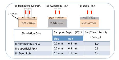
Fig. 12 Monte Carlo simulation data showing influence of PpIX depth distribution on the sampled depth of fluorescence origin and the ratio of collected light intensities. Three distributions were considered: (a) uniform PpIX throughout, (b) superficial PpIX, and (c) deep PpIX. The 80% fluorescence sampling depth is reported for blue and red excitation channels, and the red/blue ratio is given for each case.
