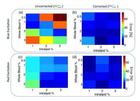
**Fig. 5** (a) and (b) The residual error between fitted PpIX fluorescence emission spectra excited by blue excitation light for uncorrected and corrected spectra, respectively. (c) and (d) The residual error between fitted PpIX fluorescence emission spectra excited by red excitation light. Residual is calculated as the percentage deviation for fitted PpIX fluorescence normalized to average of estimates from all phantoms.
