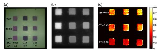
Fig. 4 Spatial mapping of quantum yield (rhodamine B): (a) white light image, (b) raw fluorescence, and (c) QY spatial mapping.
