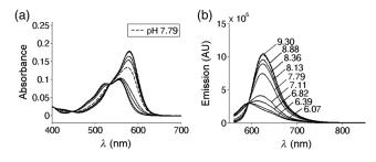
Fig. 5 SNARF-5: (a) excitation and (b) emission spectra.
