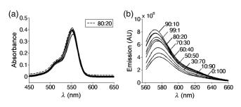
Fig. 2 Rhodamine B: (a) excitation and (b) emission spectra.
