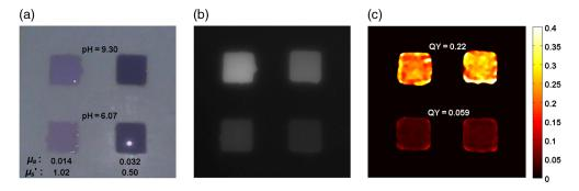
Fig. 7 Spatial mapping of quantum yield (SNARF-5): (a) white light image, (b) raw fluorescence, and (c) QY spatial mapping.
