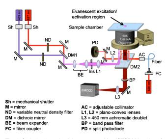
Fig. 1 Optical schematic of the setup used for dSTORM imaging of Cy5-PNA-labeled telomeres.
