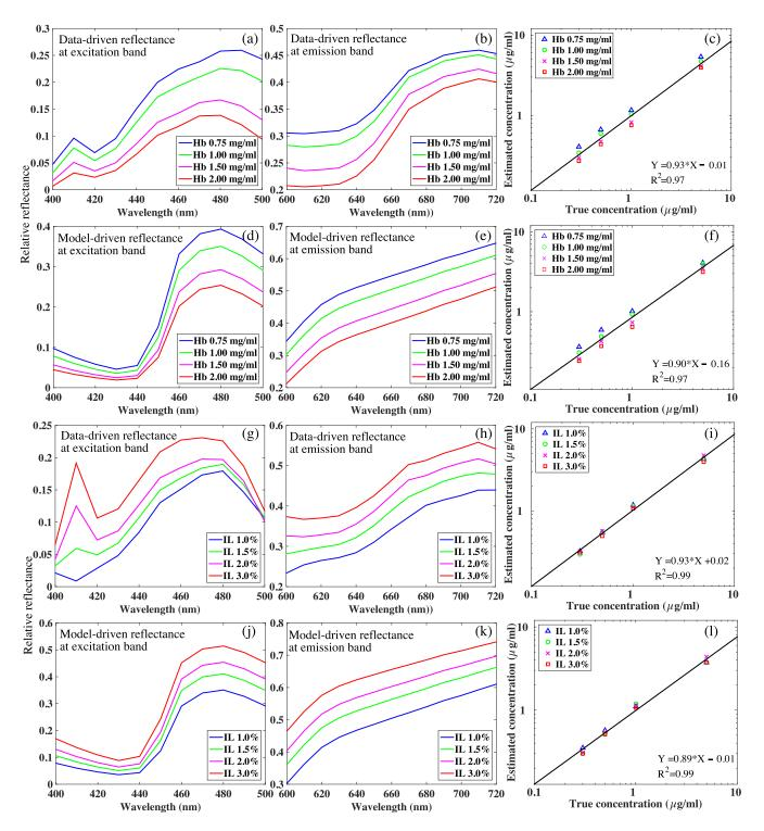
**Fig. 11** (a, b, d, e, g, h, j, k) The data-driven diffuse reflectance at both the excitation band and the emission band well correspond to the model-driven diffuse reflectance. Accordingly, (c, f, i, I) the PpIX concentrations reconstructed with the measured diffuse reflectance are consistent with the ones determined with the modeled diffuse reflectance, featuring a comparable coefficient of determination of the linear fits.
