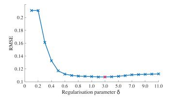
**Fig. 7** A presentative sample [the tumor specimen shown in the later figure Fig. 6(a)] demonstrating how the regularization parameter  $\delta$  is selected. RMSEs between  $C_{\text{TV}}$  and  $C_{\text{gt}}$  of different regularization parameter  $\delta$  values. The red cross marker indicates that the minimum RMSE locates at  $\delta = 3.0$ .
