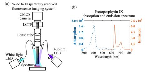
**Fig. 1** (a) Schematic of system setup and (b) the excitation and emission spectrum of PpIX (A.U.) plotted from published data.<sup>25</sup> LCTF, liquid crystal tunable filter and MO, microscope objective.
