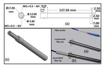
**Fig. 2** Fiber tip used for more stable measurements in different environments. (a) Dimensions of fiber tip in its top view and cross-section. (b) Fiber tip assembled with the support structure (excluding screws) to hold the fiber optic probe inside the tip. A comparison of sizes of the fiber probe with and without the tip can be made in the photograph displaying each part of the assembled fiber tip.
