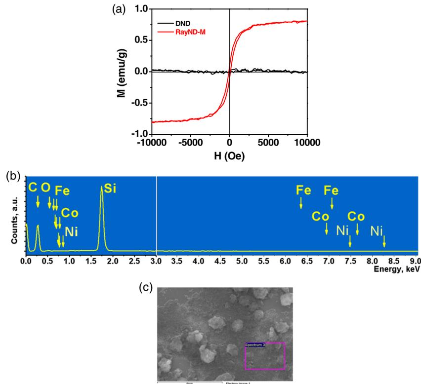
**Fig. 1** Magnetic properties of RayND-M. (a) Magnetization curve of RayND-M (I) [in comparison with ordinary DND (II)]. (b) Elemental analysis (EDX spectrum) of RayND-M. Negligible (no) containing of magnetic atoms is observed. (c) SEM image of the RayND-M powder.
