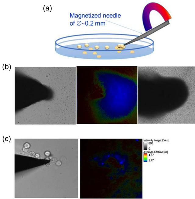
**Fig. 6** Magnetic guidance. (a) Schematic of the guidance of magnetic particles in the magnetic field. (b) Microscopic images of the needle in the RayND-M water suspension: left, the experiment beginning; center, FLIM of the particles, attracted to the needle; right, microscopic image of the needle with attracted particles after FLIM measurement. (c) RayND-M labeled A549 cells attracted to the magnetized needle: left, microscopic image and right, FLIM.
