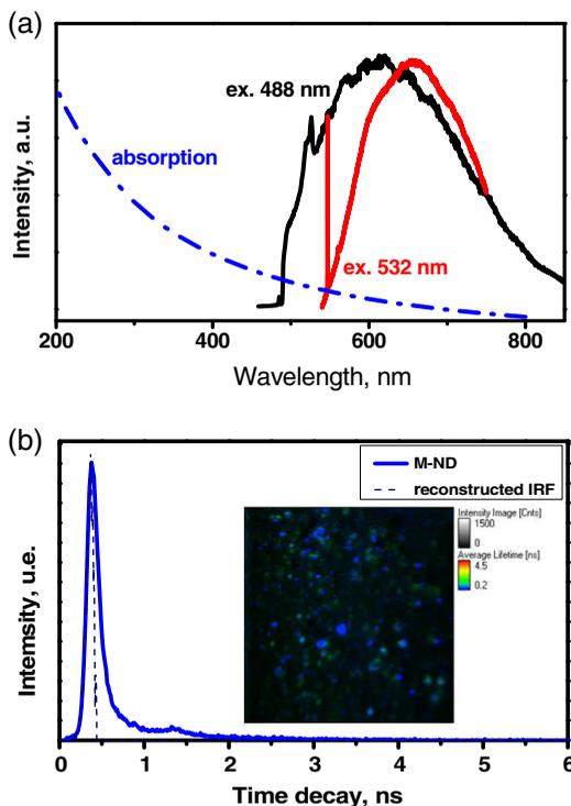
**Fig. 3** Fluorescence properties of RayND-M. (a) Absorption and fluorescence spectra at one-photon excitation; (b) lifetime decay and FLIM (inset) of RayND-M powder at two-photon excitation with femtosecond laser at 790-nm wavelength.
