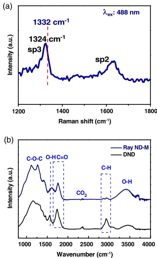
**Fig. 2** (a) Raman spectra and (b) FTIR spectra of RayND-M in comparison with DND.
