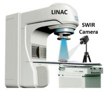
Fig. 1 Imaging setup for CESFI with an electron beam (blue).
