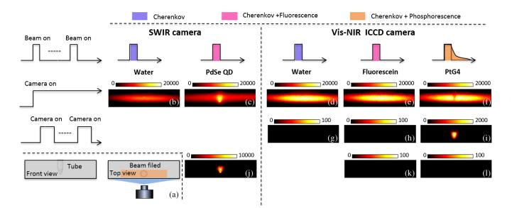
**Fig. 3** Phantom study setup and images. (a) Experimental setup. (b–f) Images obtained without timegated acquisition. (g–i) Images obtained with time-gated acquisition. (j) Image of PdSe QD by subtracting Cherenkov emission background (b) from (c). (k) Image of fluorescein by subtracting Cherenkov emission background (d) from (e). (l) Image of PtG4 by subtracting Cherenkov emission background (d) from (f).
