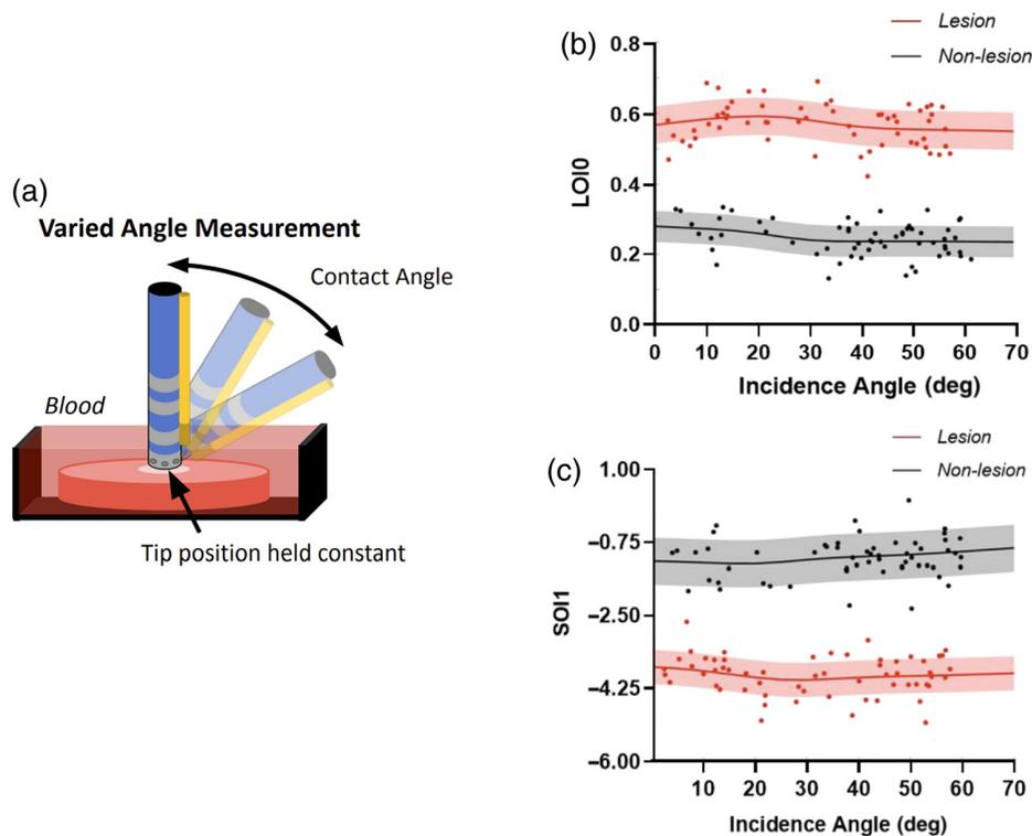
**Fig. 4** Contact angle sensitivity assessment. (a) Depiction of dedicated experiments conducted to acquire data at varying catheter contact angles, from a single location. (b) LOI<sub>0</sub> data acquired at varying contact angles on lesion and nonlesion tissue. (c) SOI<sub>1</sub> data acquired at varying contact angles on lesion and nonlesion tissue. In panels (b) and (c), lines and shaded regions illustrate sliding kernel-weighted estimates of mean and standard deviation.
