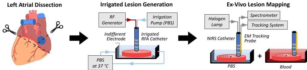
**Fig. 2** Experimental flow diagram of left atrial NIRS mapping. First, each left atrium was dissected away from the heart and flattened. Then irrigated lesions were generated in a line adjacent to a pulmonary vein. Finally, spectra were acquired from across the endocardium while the tracking system simultaneously recorded the catheter's position.
