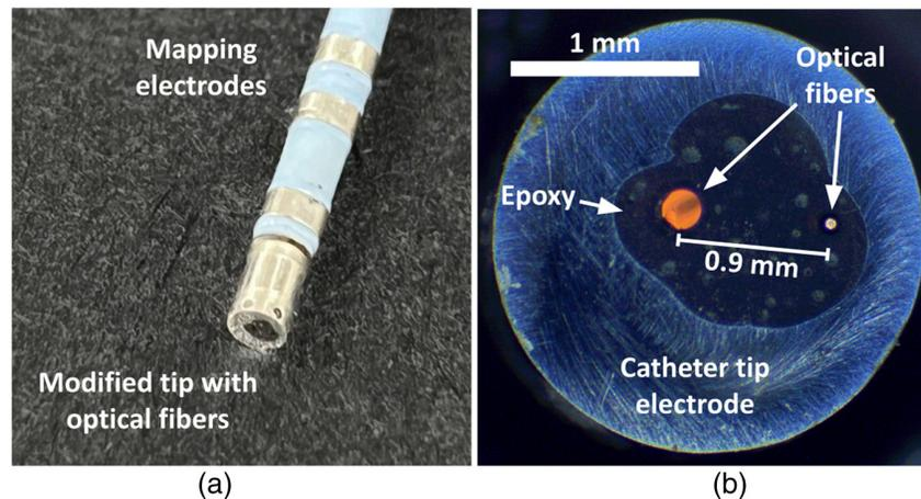
**Fig. 1** Commercial ablation catheter with integrated optical fibers for NIRS mapping. (a) Photograph of the catheter, showing the intact mapping electrodes as well as the modified tip. (b) Photomicrograph of the catheter tip illustrating the positions of the two multimode optical fibers.
