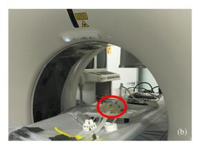
**Fig. 4** Benchtop setup of 3D printed patient-specific phantoms. (a) Phantoms in established flow loop with programmable pulsatile pump with pressure sensors attached and (b) phantom, outlined in red, in Aquilion ONE scanner for CCTA scans.
