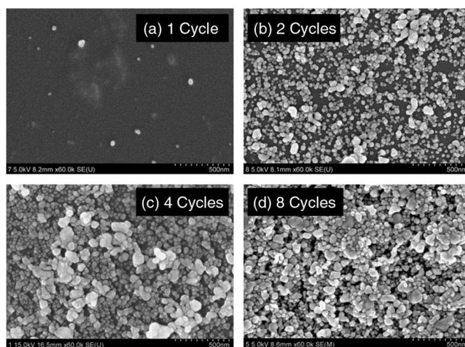
**Fig. 2** Scanning electron microscope (SEM) images for Ag NPs prepared by (a) one, (b) two, (c) four, and (d) eight deposition cycles.
