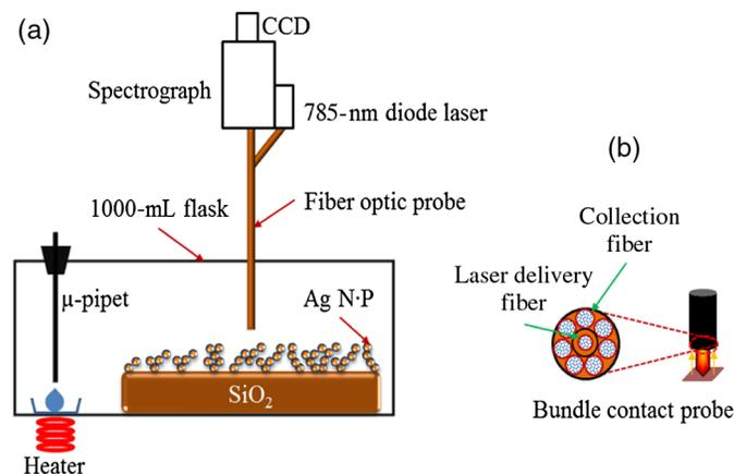
**Fig. 1** Schematic view of surface-enhanced Raman scattering (SERS) measurement of organic vapors. A 1000-mL volumetric flask (a) and an optical-fiber bundle comprising one core excitation fiber and seven surrounding collection fibers (b) are used. The excitation wavelength and intensity was 785 nm and 15 mW, respectively.
