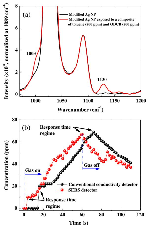
**Fig. 5** (a) Raman spectra for a composite vapor comprising toluene (at 200 ppm) and ODCB (at 200 ppm) (red) and for a reference SERS substrate (black). (b) Data for a real-time monitoring of flowing toluene vapor, obtained by SERS detector (red) and conventional conductivity detector (black).
