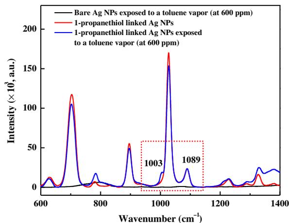
**Fig. 3** Raman spectra for bare Ag NPs exposed to a toluene vapor (black, at 600 ppm), 1-propanethiol linked Ag NPs (red), and 1-propanethiol linked Ag NPs exposed to a toluene vapor (blue, at 600 ppm). Baselines were consistently subtracted from the Raman spectra using a polynomial function.
