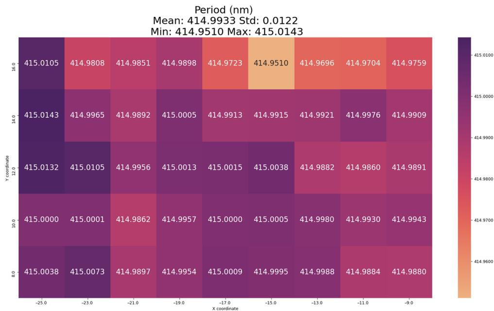
**Fig. 8** Example of outcoupler grating period uniformity for one sample.
