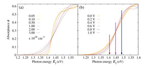
**Fig. 2** The strong built-in potential present in the ultra-thin junction leads to a Franz–Keldysh tailing of the band edge, inducing the absorption of sub-bandgap energy photons. Following the strength of the built-in field, the tailing (a) increases with doping density and (b) decreases with forward bias. The effect on the absorptance depends on the photon energy, whereas the absorption is increased at sub-bandgap energies, it is reduced above the band edge.
