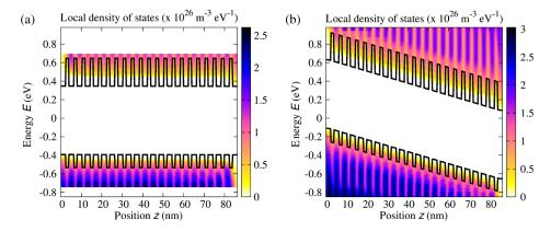
**Fig. 6** Local density of states of a 20-period quantum well superlattice at vanishing bias voltage and (a) flat band conditions, corresponding to an intrinsic system, and (b) for a doping density of  $2 \times 10^{18}$  cm<sup>-3</sup>. Although the effective bandgap is increased as compared with bulk InGaAs because of confinement, the strong coupling results in a pronounced carrier delocalization and associated quasi-3D DOS.
