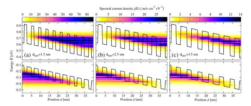
**Fig. 9** Photocurrent spectrum (0.1 kW/cm<sup>2</sup>@0.95 eV) of coupled quantum well absorber structures with fixed InGaAs QW size of 2.5 nm and InAlGaAs layer thicknesses ranging from 1.5 to 3.5 nm. With increasing barrier width, the character of carrier transport gradually changes from quasi-ballistic to phonon-assisted sequential tunneling.
