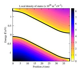
**Fig. 1** Band profile and local density of states of a 40-nm GaAs *pin* junction solar cell. The doped layers extend over 10 nm and provide a charge carrier density of  $3 \times 10^{18}$  cm<sup>-3</sup>.
