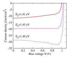
Fig. 3 The bias dependence of the absorptance at different photon energies as displayed in Fig. 2 is reflected in the monochromatic current–voltage characteristics (@0.1 kW/cm²).
