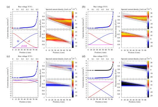
**Fig. 8** JV characteristics, integral and spectral current flow at (a) short-circuit conditions (0 V), (b) close to the maximum power point (0.45 V), (c) at open-circuit conditions (0.52 V), and (d) at open-circuit voltage in the dark. Although the minibands break up under realistic built-in fields, carrier extraction proceeds almost ballistically for thin barriers.
