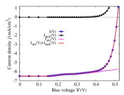
**Fig. 7** Current voltage characteristics of the 20-period superlattice in the dark and under monochromatic illumination with photons of 0.95 eV and at 0.1 kW/cm<sup>2</sup>. Because of the high degree of delocalization, the carrier escape probability is unity, i.e., the light JV-curve is the exact superposition of the bias-dependent photocurrent from the absorptance and the radiative dark current.
