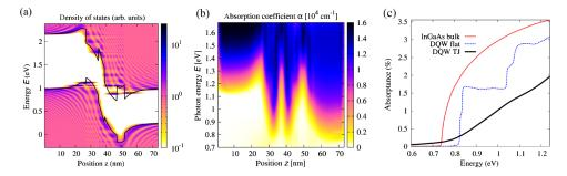
**Fig. 10** (a) Local density of states in a double quantum well tunnel junction, (b) associated local absorption coefficient, and (c) the overall absorptance of the structure, revealing pronounced deviations from the flat band situation of a square well potential and bulk injection regions.
