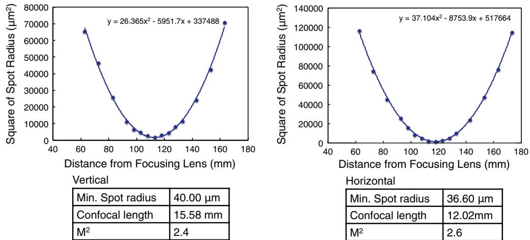
Fig. 6  $M^2$  measurement results for the output FHG beam.
