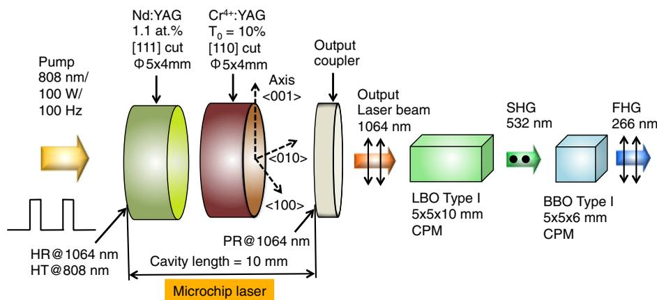
Fig. 1 Laser configuration with no intervening optics before nonlinear crystals.
