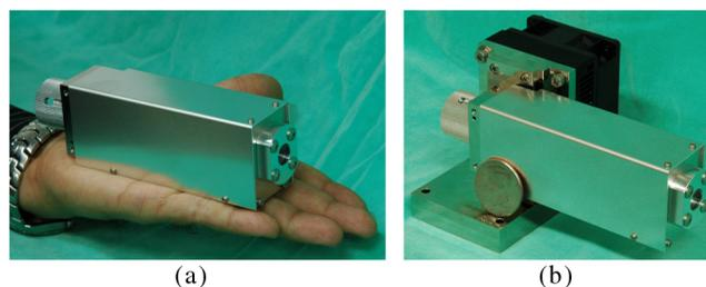
Fig. 2 Photograph of microlaser prototype without cooling (a) and with thermoelectric cooling (b).
