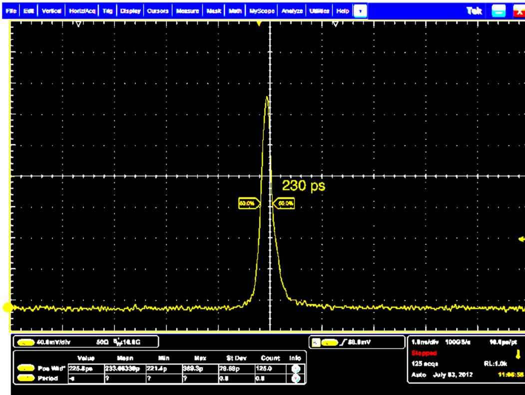
**Fig. 3** Temporal profile of the fundamental laser output having a pulse width of 230 ps, measured using Tektronix DPO71604C oscilloscope and EOT ET-3500 detector.
