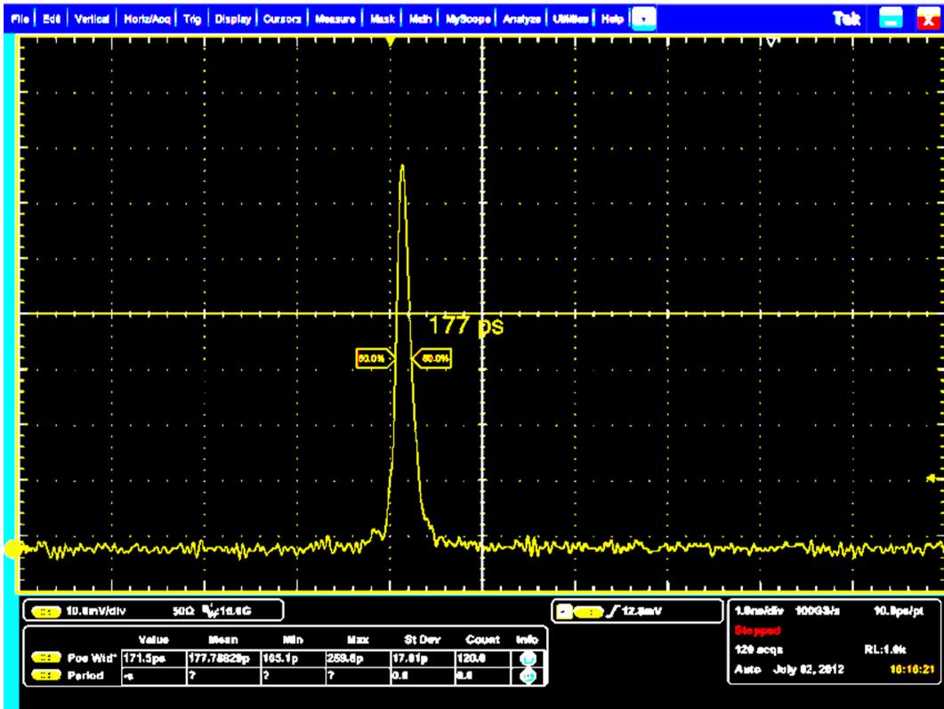
Fig. 4 Temporal profile of SHG output having a pulse width of 177 ps, measured using Tektronix DPO71604C oscilloscope and EOT ET-4000 detector.
