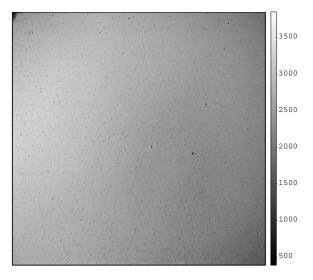
**Fig. 7** Flat-field illumination of H1RG-16885 through a circular variable filter wheel centered at 5.6  $\mu$ m. The dark spots with bright halos are diffraction/shadows from dust specks suspended 800  $\mu$ m in front of the detector surface, demonstrating the good imaging properties of the array.
