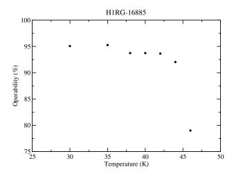
Fig. 4 Operability versus focal plane temperature for H1RG-16885.
