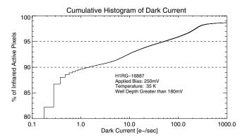
Fig. 11 Histogram of the cumulative dark current for H1RG-16887 for well depths >180 mV for 250 mV reverse bias at a focal plane temperature of 35 K. Only infrared active pixels are included.
