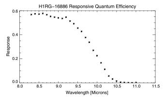
Fig. 8 Responsive quantum efficiency (RQE) as a function of wavelength for H1RG-16886 at a focal plane temperature of 35 K.
