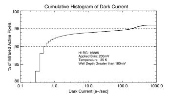
Fig. 3 Histogram of the cumulative dark current for H1RG-16885 for well depths >180 mV for 200 mV reverse bias at a focal plane temperature of 35 K. Only infrared active pixels are included.
