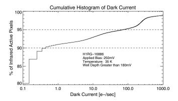
**Fig. 9** Histogram of the cumulative dark current for H1RG-16886 for well depths >180 mV for 250 mV reverse bias at a focal plane temperature of 35 K. Only infrared active pixels are included.
