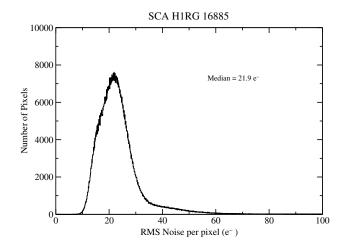
**Fig. 6** Histogram of Fowler-1 noise/pixel for H1RG-16885. Fowler-1 sampling is equivalent to correlated double sampling.
