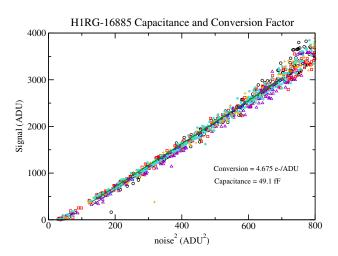
Fig. 1 Capacitance per pixel determined for H1RG-16885, with no IPC (interpixel capacitance) correction applied.
