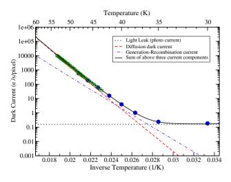
Fig. 5 An Arrhenius plot of dark current per pixel versus inverse temperature for an actual well depth (reverse detector bias) of 240 mV.
