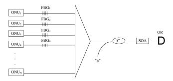
Fig. 1 Fiber laser sensor is utilized to monitor the fiber faulty of treestructured PON. OR is the optical reflector, C is the bidirectional 3-dB Coupler, OLT is the optical line terminator, and ONU is the optical network unit. The OSA is placed at point "a."<sup>16</sup>
