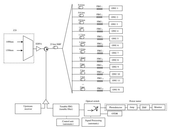
Fig. 4 Block diagram of time division multiplexing (TDM)-PON monitoring system. SMF is the single-mode fiber and ONU is the optical network unit.
