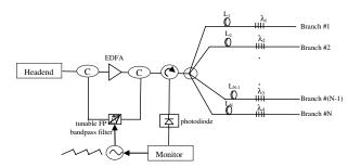
Fig. 3 Fiber fault monitoring scheme for an optical amplified branched network.<sup>18</sup>
