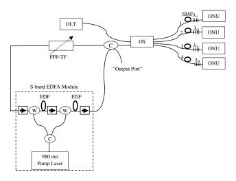
**Fig. 2** Experimental setup of the proposed S-band erbium-doped fiber (EDF) laser scheme for monitoring the fiber fault in passive optical networks (PONs).<sup>17</sup>
