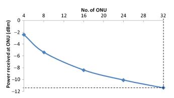
Fig. 9 The received downstream signal power versus number of ONUs.
