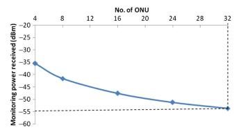
Fig. 8 The received monitoring power that is measured using a power meter versus number of ONUs.
