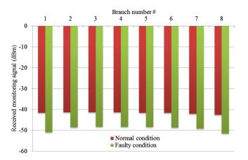
Fig. 6 The received monitoring signal at the specific branch during normal condition and when there is a fault in the network.
