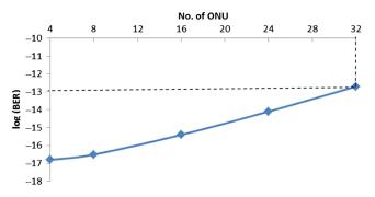
Fig. 7 Bit error rate (BER) versus number of ONUs with the monitoring system.
