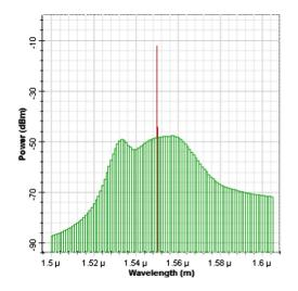
Fig. 5 The amplified spectrum of 1550-nm downstream signal.
