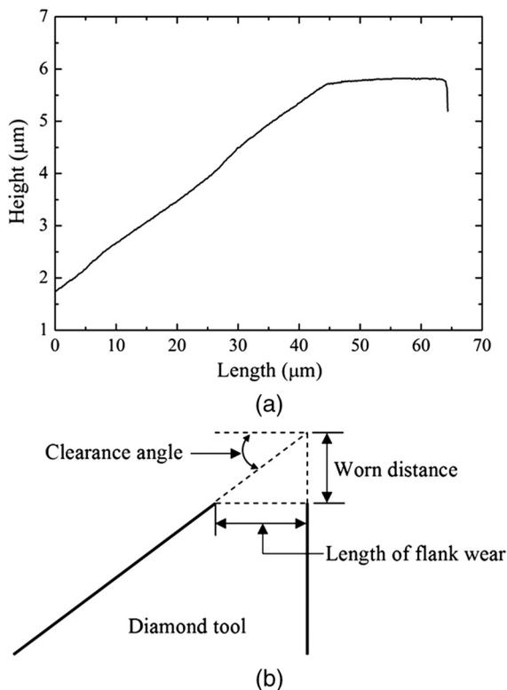
**Fig. 7** Measured profile of the flank face (a) and tool geometry (b).
