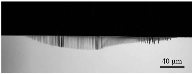
**Fig. 6** Wear for a single-crystal diamond tool with a 3 mm nose radius. The tool was used under mixed feed rates of 1 and 2  $\mu\text{m}/\text{rev}$  during machining the electroless nickel. The grooves on the flank face are not clear.
