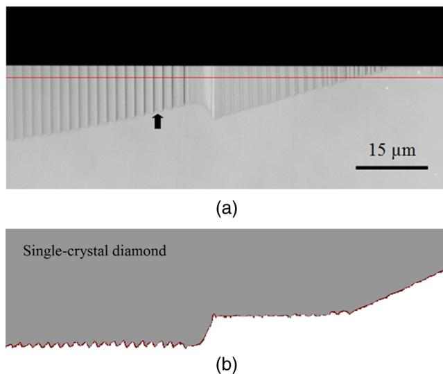
**Fig. 4** Measured line profile for the defect on the diamond tool after machining electroless nickel. The line profile (b) corresponds to the line in (a). Cutting direction is from left to right in (a) and (b).
