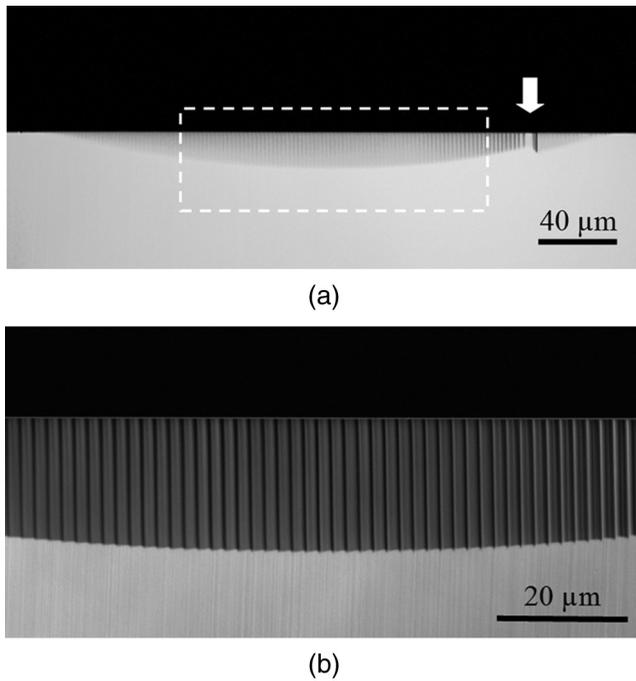
**Fig. 3** Flank face of the worn diamond tool with a 5 mm nose radius after machining electroless nickel for a 3.18-km distance. Cutting direction is from left to right in (a).
