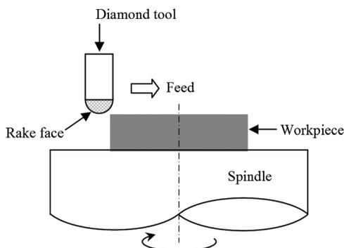
Fig. 1 Single-point diamond turning of electroless nickel.
