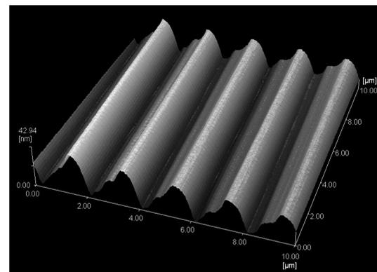
**Fig. 5** Flank face (measured with the SPM) of the worn diamond tool after electroless nickel turning.
