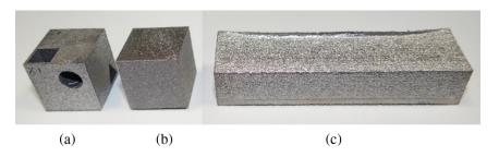
Fig. 1 Pictures of the samples: (a) Al-Si-10Mg, (b) Ti-6Al-4V LPBF cubes, and (c) Ti-6Al-4V EBPBF rectangular prism.
