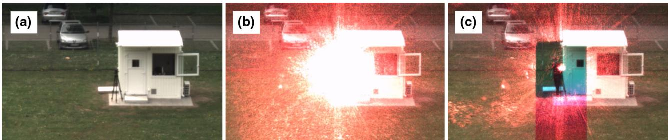
**Fig. 8** Images taken at a field trial with the hardened sensor: (a) scene without disturbing laser radiation, (b) scene with laser dazzle; the protection measure (DMD) was not activated, (c) scene with laser dazzle; the protection measure (DMD) was activated.
