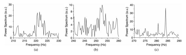
**Fig. 5** Power spectra for probe beams consisting two LG lights of (a)  $l = \pm 7$ , (b)  $l = \pm 8$ , and (c)  $l = \pm 9$ . The corresponding beat frequencies are 221.9  $\pm$  1.7 Hz, 252.5  $\pm$  0.8 Hz, and 284.1  $\pm$  0.2 Hz (measured as FWHM).
