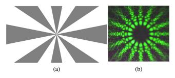
Fig. 3 (a) Phase profile of LG  $\pm 8$  modes and (b) corresponding far-field intensity profile.
