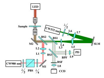
**Fig. 2** The experimental setup used for the rotational Doppler effect. Labels denote the continuous wave (CW), half-wave plate ( $\lambda/2$ ), polarizing beam splitter (PBS), quarter-wave plate (I/4), mirror (M), lenses (L), beam splitter (BS), SLM, bandpass filter (BPF), bandstop filter (BSF), and photodiodes (PD)
