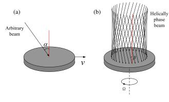
Fig. 1 (a) Linear Doppler effect and (b) rotational Doppler effect.
