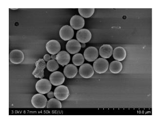
Fig. 4 SEM image of the silk fibroin regulated vaterite microspheres.
