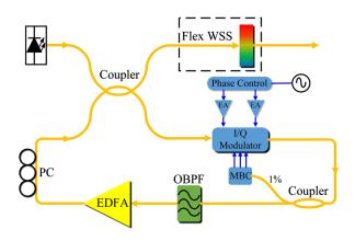
Fig. 6 Experimental setup of the proposed dynamic RFS.
