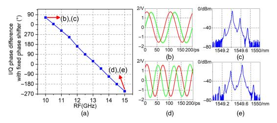
**Fig. 3** I/Q phase difference and optical spectrum using fixed phase shifter: (a) I/Q phase difference when RF frequency changes from 10 to 15 GHz, (b) RF time-domain signal at 10 GHz, (c) optical spectrum after first RT at 10 GHz, (d) RF time-domain signal at 15 GHz, and (e) optical spectrum after first RT at 15 GHz.
