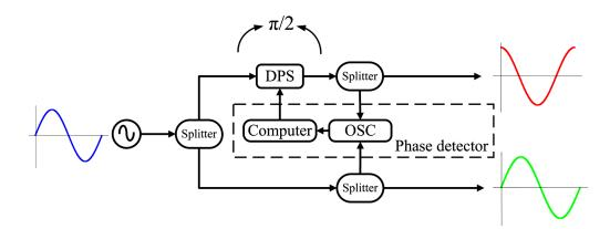
Fig. 4 Structure of the phase control module.
