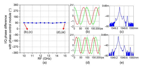
Fig. 5 I/Q phase difference and optical spectrum with phase control module: (a) I/Q phase difference when RF frequency changes from 10 to 15 GHz, (b) RF time-domain signal at 10 GHz, (c) optical spectrum after first RT at 10 GHz, (d) RF time-domain signal at 15 GHz, and (e) optical spectrum after first RT at 15 GHz.
