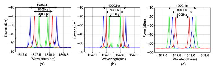
Fig. 9 Optical spectrum after WSS with RF set to: (a) 10 GHz, (b) 12.5 GHz, and (c) 15 GHz.
