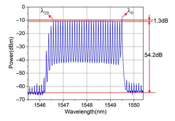
Fig. 7 30 stable frequency-locked-carrier spectrum with 12.5-GHz interval.
