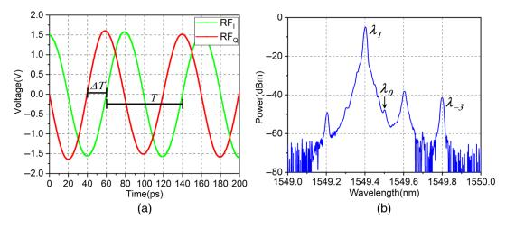
Fig. 2 When  $\theta$  is equal to  $\pi/2$  and RF is 12.5 GHz: (a) RF time-domain signal and (b) optical spectrum after the first RT.
