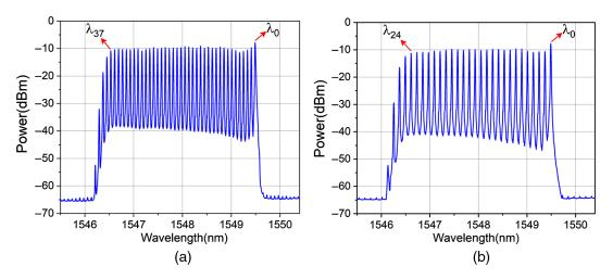
Fig. 8 Multicarrier generation with: (a) 10-GHz interval and (b) 15-GHz interval.
