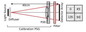
Fig. 2 Experimental layout for the calibration polarization state generator and the microgrid polarization camera. A diffuser is used to ensure that the light source is unpolarized. The inset at right shows a  $2 \times 2$  section of the detector array.
