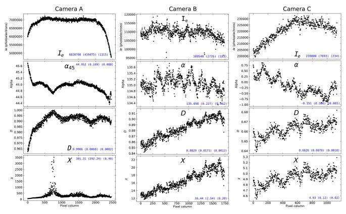
**Fig. 6** Parameter estimates for a row through the camera images, calculated after summing 2000 frames for camera A, 100 frames for cameras B and C. The inset numbers give the measured mean and standard deviation, and the theoretical noise-only standard deviation, of the row data.
