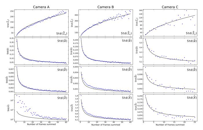
**Fig. 5** Temporal standard deviation of each parameter for a single pixel in each camera. The horizontal axis indicates the number *N* of frames summed prior to calculating the parameter standard deviation. The dots indicate measurements, whereas the curve indicates the theoretical standard deviation value calculated from the measured light level. Note that the camera A subfigure for  $\hat{X}$  uses a semilogarithmic plot, while all of the other subfigures use a linear plot.
