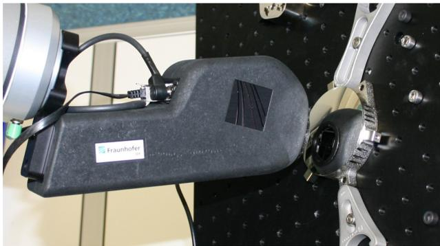
**Fig. 10** Full-surface roughness and defect assessment using a light scattering sensor: photography of robot-guided scattering sensor and the sample.
