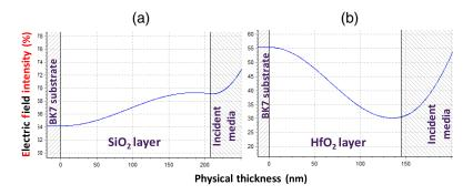
**Fig. 2** Electric field calculations in (a)  $SiO_2$  and (b)  $HfO_2$  single layers at 0° of AOI, P or S polarizations. The EFI is maximum at the top of the  $SiO_2$  layer (at the air interface and its value is 69.9%) and maximum at the bottom of the  $HfO_2$  layer (at the substrate interface and its value is 54.6%).
