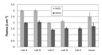
**Fig. 3** Histogram of intrinsic LIDTs on each laboratory for  $SiO_2$  and  $HfO_2$  single layers. The last two bars correspond to the averages of the different installations. Vertical lines are error bars.
