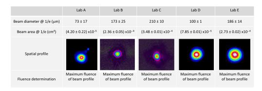
Fig. 5 Laser beam sizes and spatial for the five facilities.
