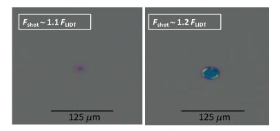
Fig. 1 Post-mortem observation by means of a Nomarski microscope for two irradiations on  $HfO_2$  at 10% and 20% above  $LIDT_{exp}$ .
