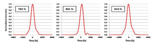
Fig. 4 Three different temporal profiles measured during the campaign at Lab B by means of SPIRITED diagnostic, for the same laser fluence.
