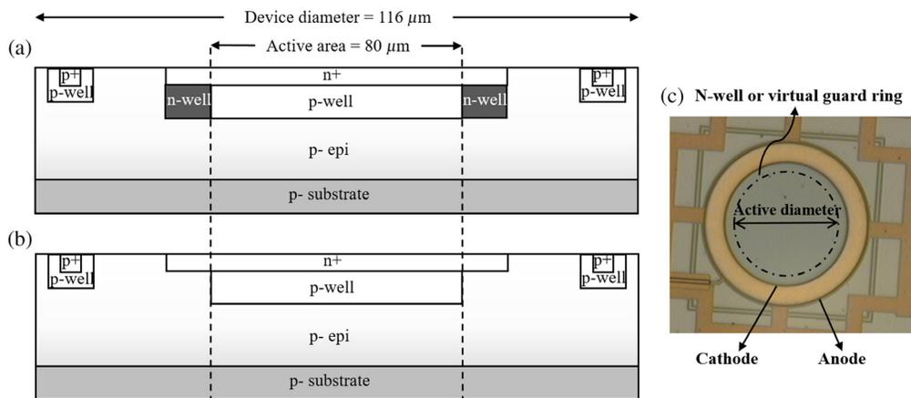
**Fig. 1** Schematic cross-section (not to scale) of CMOS SPADs based on n<sup>+</sup>/p-well structure with (a) the physical guard ring (SPAD1) and (b) the virtual guard ring (SPAD2). (c) Top view of these SPADs (there is no difference in the chip photos of both SPADs visible).
