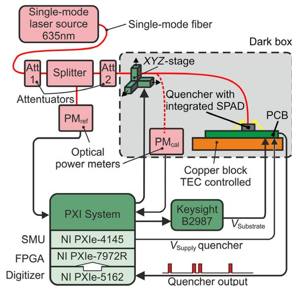
Fig. 2 Schematic of the measurement setup.
