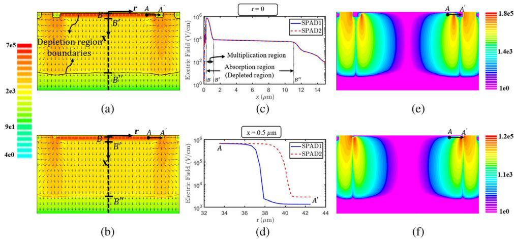
**Fig. 3** 2D plots of the electric field obtained by TCAD simulation for (a) SPAD1 and (b) SPAD2 in logarithmic scale. Arrows indicate the local electric field direction. (c) A vertical cross-section of the electric field at the center ( $r = 0$ ) for both SPAD1 and SPAD2. (d) A lateral cross-section of the electric field through  $A-A'$  at  $x = 0.5 \mu\text{m}$  in SPAD1 and SPAD2. 2D plots of the  $r$ -component of the electric field for (e) SPAD1 and (f) SPAD2 in logarithmic scale.
