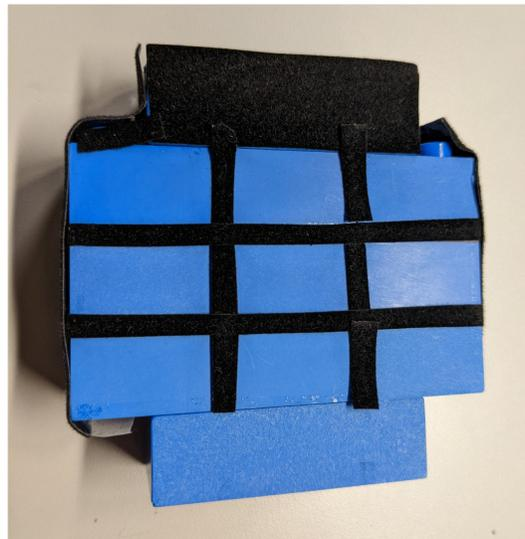
**Fig. 2** A tower of blue plastic LEGO bricks, each being sanded with a different grit of sandpaper. This represents a group of objects with similar properties and albedos for a given wavelength but with different surface textures. The  $Ra$  in microns for each brick are top: 0.49, 0.56, 3.35, middle: 3.55, 2.62, 0.35, and bottom: 1.68, 1.26, 6.32.
