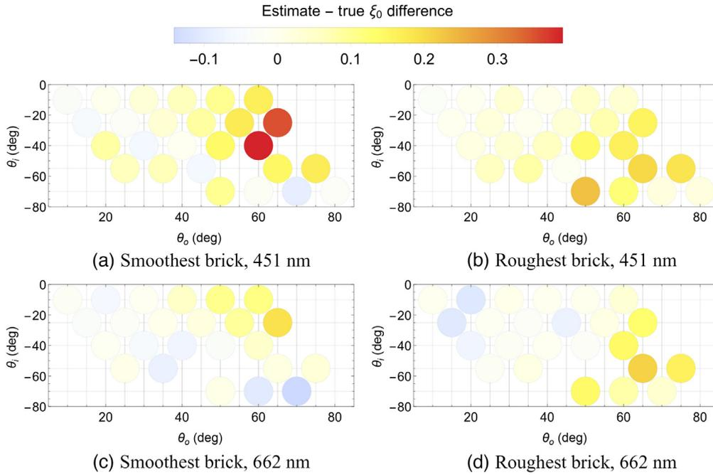
**Fig. 5** The estimate  $\tilde{\xi}_0$  calculated with Eq. (14) minus the true  $\xi_0$  versus acquisition geometry at 451 nm for (a) the smoothest brick and (b) the roughest brick, and at 662 nm for (c) the smoothest brick and (d) the roughest brick. When the difference is positive valued, the contribution of the dominant non-depolarizing term is overestimated. Geometries at which the dynamic range of the linear Stokes camera caused non-physical MM extrapolations are omitted.
