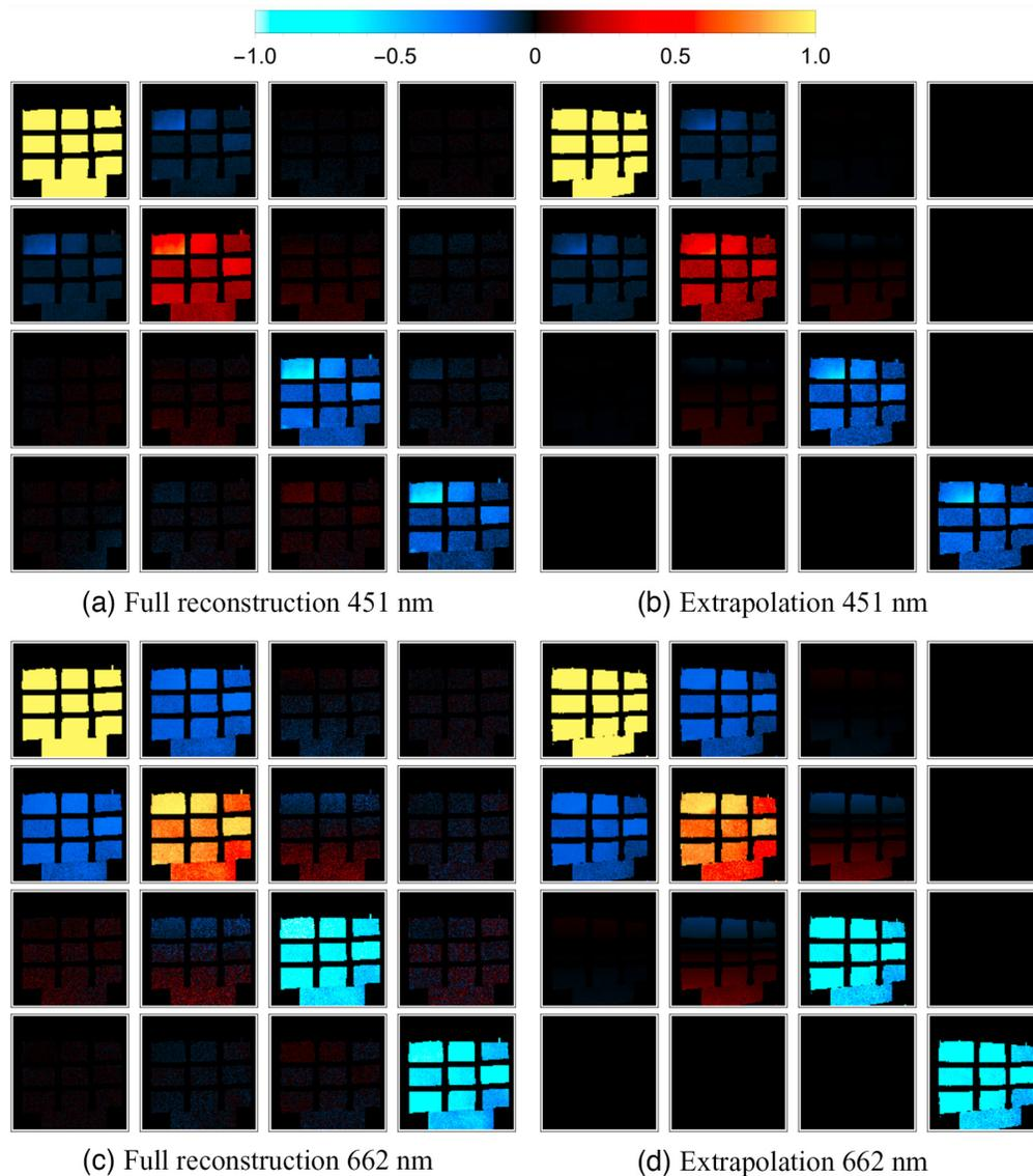
**Fig. 3** Comparison of the MM image results at 451 nm of (a) full reconstruction with 40 polarimetric measurements to (b) MM image results of partial polarimetric extrapolation (Video 1) and at 662 nm of (c) full reconstruction and (d) extrapolation (Video 2). The still images are for the geometry  $\theta_i = -25$  deg,  $\theta_o = 25$  deg (Video 1, MP4, 3 MB [URL: <https://doi.org/10.1117/1.OE.61.12.123104.s1>]; Video 2, MP4, 4 MB [URL: <https://doi.org/10.1117/1.OE.61.12.123104.s2>]).
