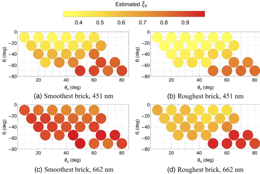
**Fig. 4** The estimate  $\tilde{\xi}_0$  calculated with Eq. (14) versus acquisition geometry at 451 nm for (a) the smoothest brick and (b) the roughest brick, and at 662 nm for (c) the smoothest brick and (d) the roughest brick. Geometries at which the dynamic range of the linear Stokes camera caused non-physical MM extrapolations are omitted.
