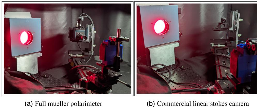
**Fig. 1** (a) The full Mueller imaging polarimeter referred to as the RGB950. It takes 40 polarimetric measurements. (b) The goniometer and PSG of the RGB950 but with the PSA replaced by a commercial off-the-shelf linear Stokes camera. The Stokes camera takes 4 polarimetric measurements in a single snapshot with a static PSG state.
