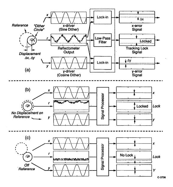
Fig. 3 Generation of analog tracking feedback signals from a confocal reflectometer.
