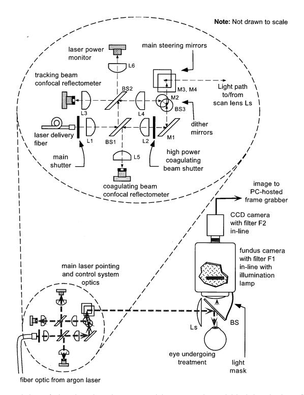
Fig. 4 Optical schematic for the analog tracking technique. An expanded view is inset to show needed detail. The tracking beam reflectometer detects the dither signal and the coagulating beam reflectometer is used to control therapeutic lesion formation. Main beam steering mirrors: M3 and M4. Dithering performed by M2 and BS3.
