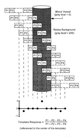
Fig. 1 Response of a 1-D template in the vicinity of a blood vessel.
