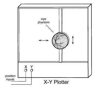
**Fig. 6** Illustration of an eye phantom attached to the pen holder armature of an XY plotter to produce simulated eye movements.
