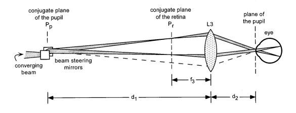
Fig. 5 The light path of the analog tracking setup shows how incident and reflected light of the tracking and coagulating beams is coupled into and out of the eye. Not drawn to scale.
